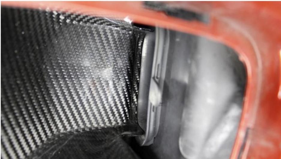
58. The rear part of the scoop should sit inside the stock duct opening, this side can get caught at the bottom of the stock duct, align as shown.
