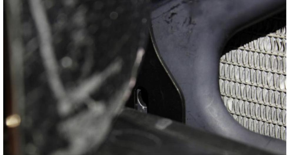
54. The bracket should line up with the hole in the strut brace as shown.
