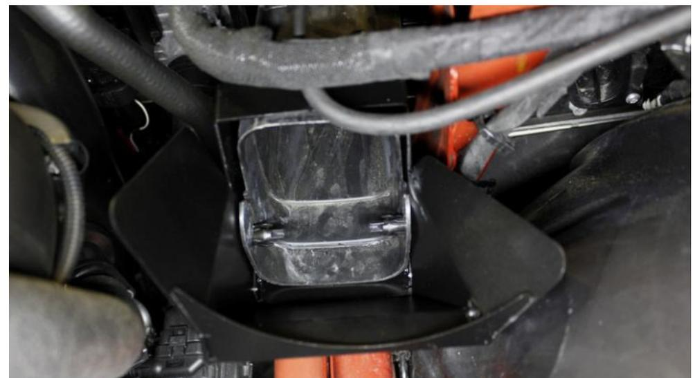
27. Use the 2 push rivets to again secure the duct in place. Press the rivet heads in fully to lock. Again, there will be some movement in the duct - which is required.
