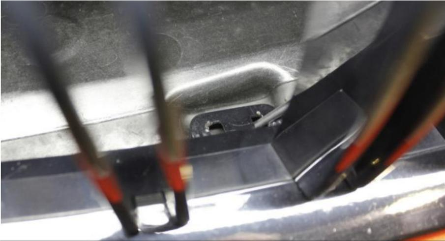
47. Remove the front grills. There are 8 tabs per grill – see next photo. The lower tabs need to be pulled up and the upper tabs to be pulled down. Start with the lower tabs - use a small screwdriver passed behind the grill to pull the centre of the tabs up. Pull the grill towards as you do this to release it. Once the lower tabs are released, use your fingers to pull the upper and side tabs down. Again – do this while pulling on the grill.
