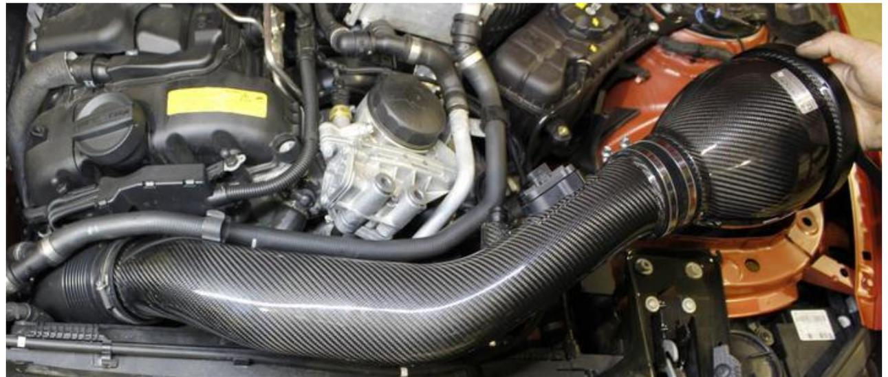
38. Lower the assembly into the engine bay – locate the carbon tube into the stock intake tube and push in.
