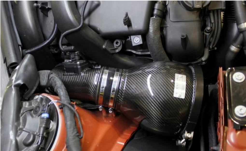
36. Finally – reconnect the MAF sensor plug – there should be enough slack in the loom from removing it from the clip earlier. Ensure the connector is clicked in all the way. Tighten the Band Clamp holding the housing and filter together.
