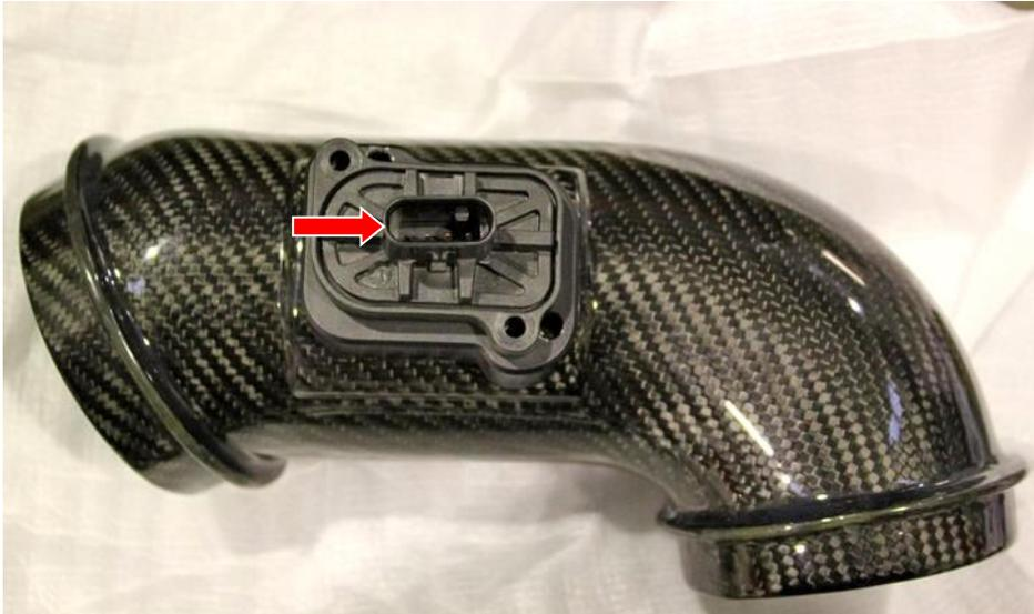
17. Insert MAF sensor into LHS tube – **ensure that the sensor is oriented correctly**. There is an arrow on the sensor indicating direction of airflow which is highlighted here in red.
