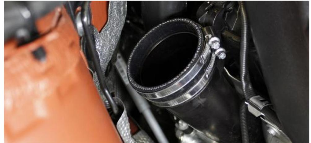
29. Taking the shorter 76mm coupler, push over the intake tube on the LEFT side of the engine. Make sure the coupler is pushed down fully and put two hose clamps around the coupler as shown. Tighten the LOWER clamp only.
