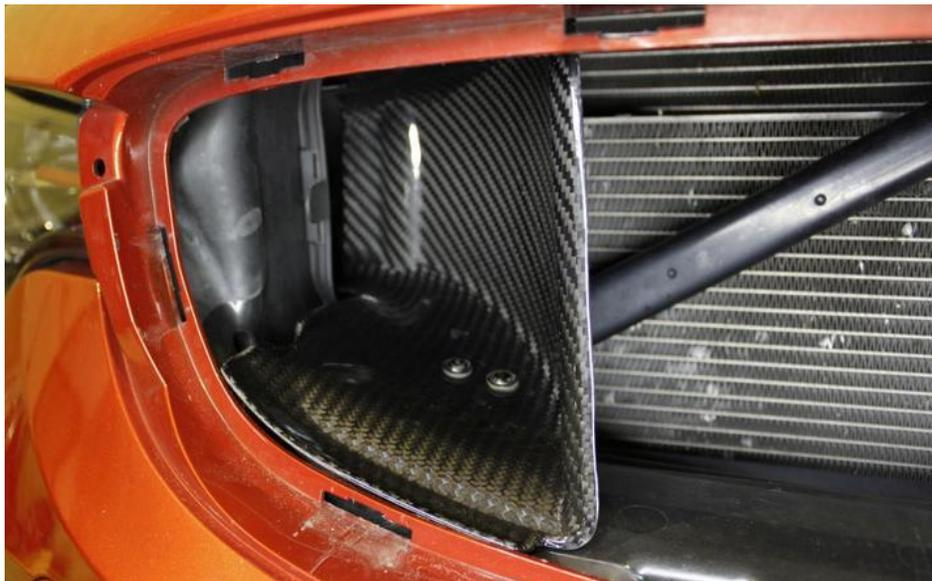
52. The scoop should be as shown with the lower lip against the top of the grill panel.
