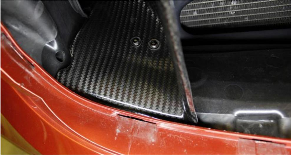
53. Now pull the bumper area at the bottom of the grill out to allow the lower lip of the scoop to locate underneath.
