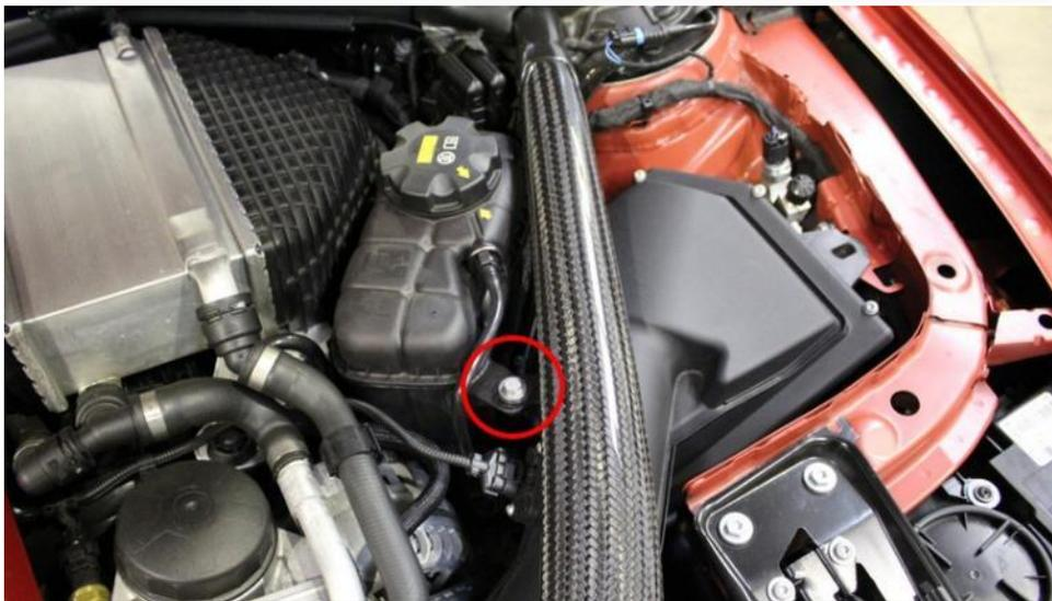
3. Remove the 10mm bolt secured to the coolant tank.
