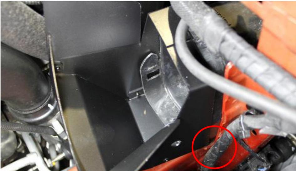
26. Locate the left duct onto the stock opening. The stock plastic opening should go INSIDE the new duct. The left corner can get obstructed by the chassis metal work circled here – avoid contact and locate the holes.
