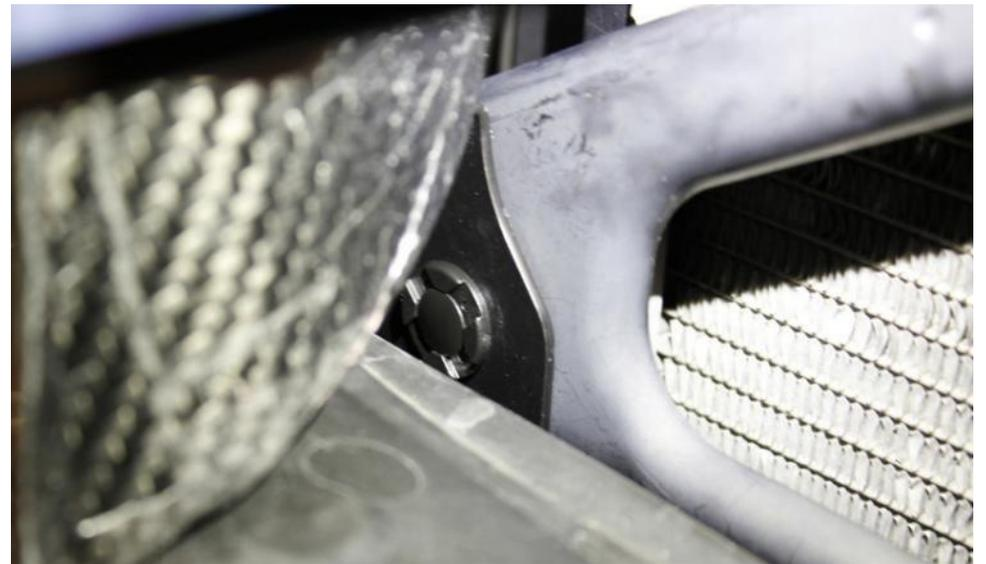
56. Push rivet fully secured in place.
