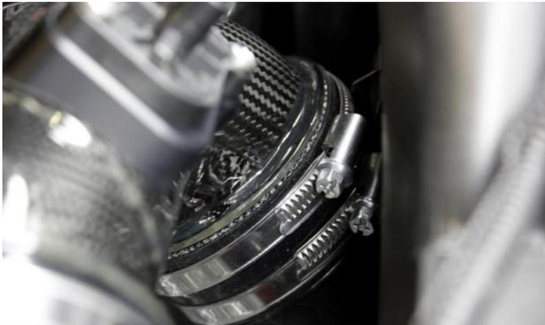
34. Push the tube all the way into the silicon so that the flange on the tube meets the silicon all the way around. Don't tighten yet.
