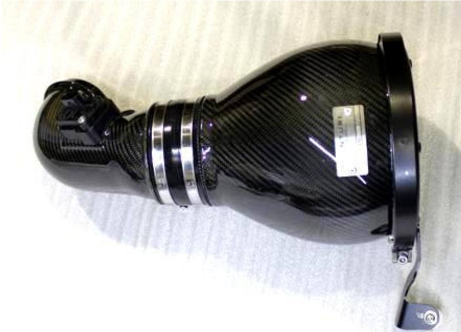
32. Orient the tube as shown. Tighten Hose clamp on the housing, leave the clamp on the tube loose enough to allow the tube to still be rotated.
