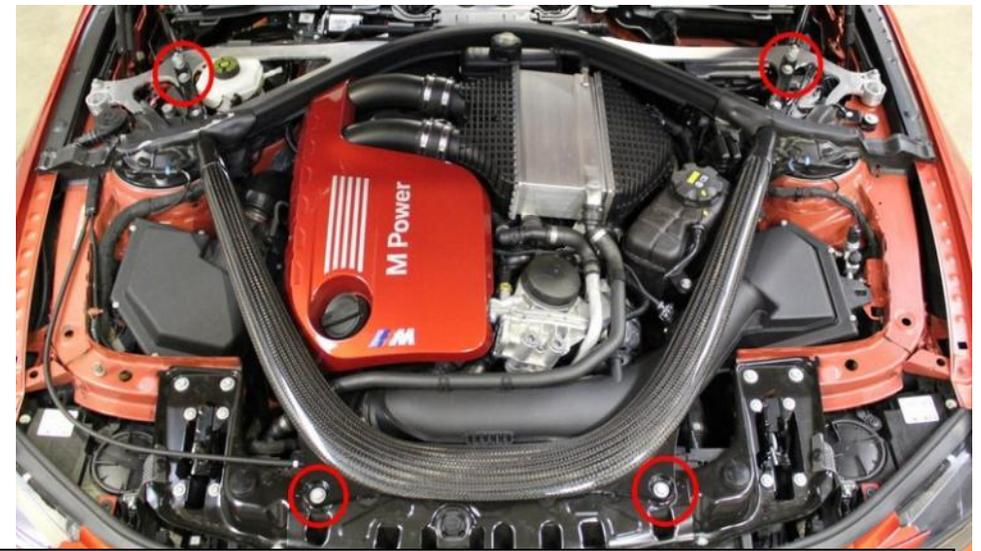
2. Remove the 8 13mm bolts holding the strut brace down. There is also a 10mm bolt secured to the coolant tank – see next photo.
