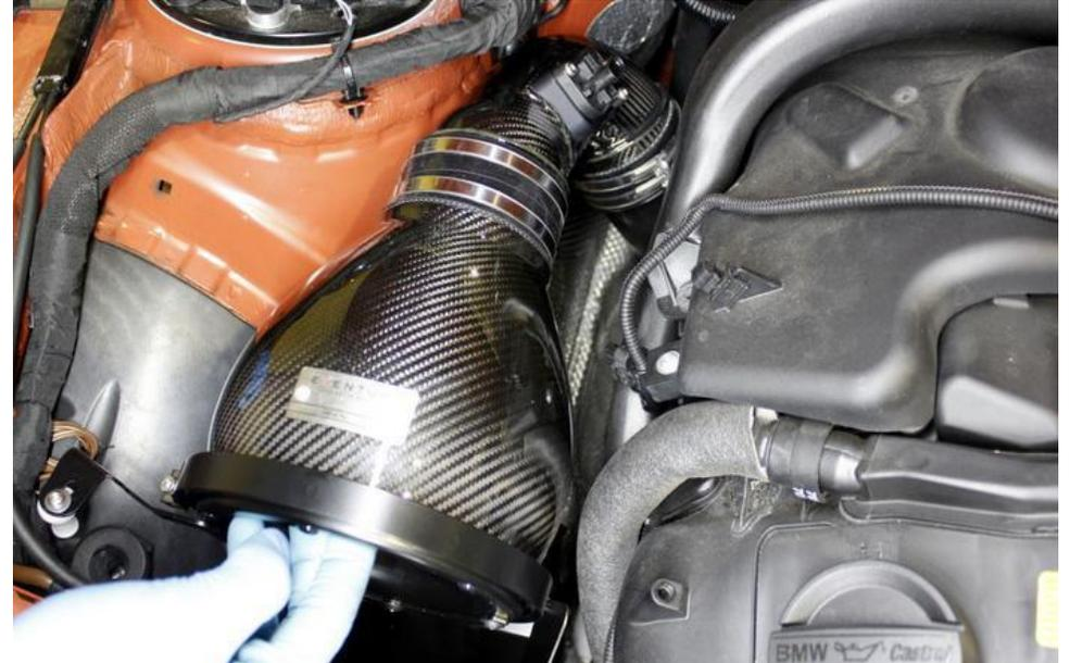
33. Lower the intake assembly into the left side and push the tube into the silicon coupler installed previously. Locate the opening of the intake into the duct installed previously. Rotate band clamp if needed for clearance with duct – see step 35.
