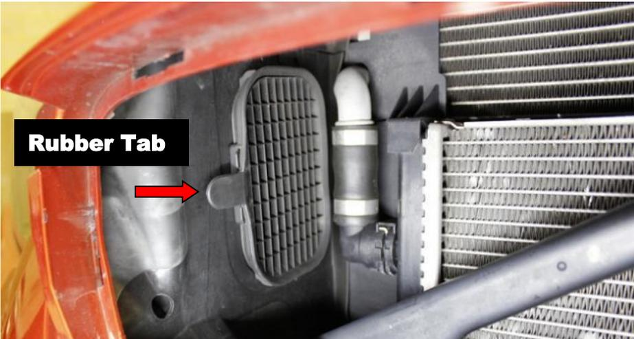
48. With the grills removed, you will see these inner grids which need to be removed. Simply pull the rubber tab to release the grid and remove completely. See next photo.
