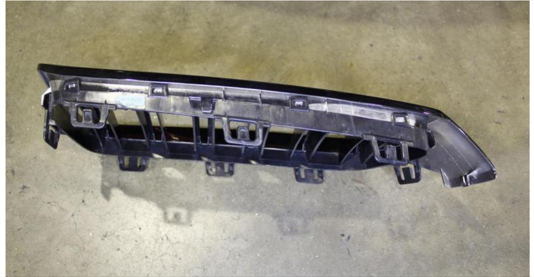
Here is the removed grill with tabs shown. If you cannot release the tabs as shown, you will need to remove the Torx screws holding the top of the bumper in. They are under the rubber strip. You can then pull the top of the bumper out and gain access from the top.
