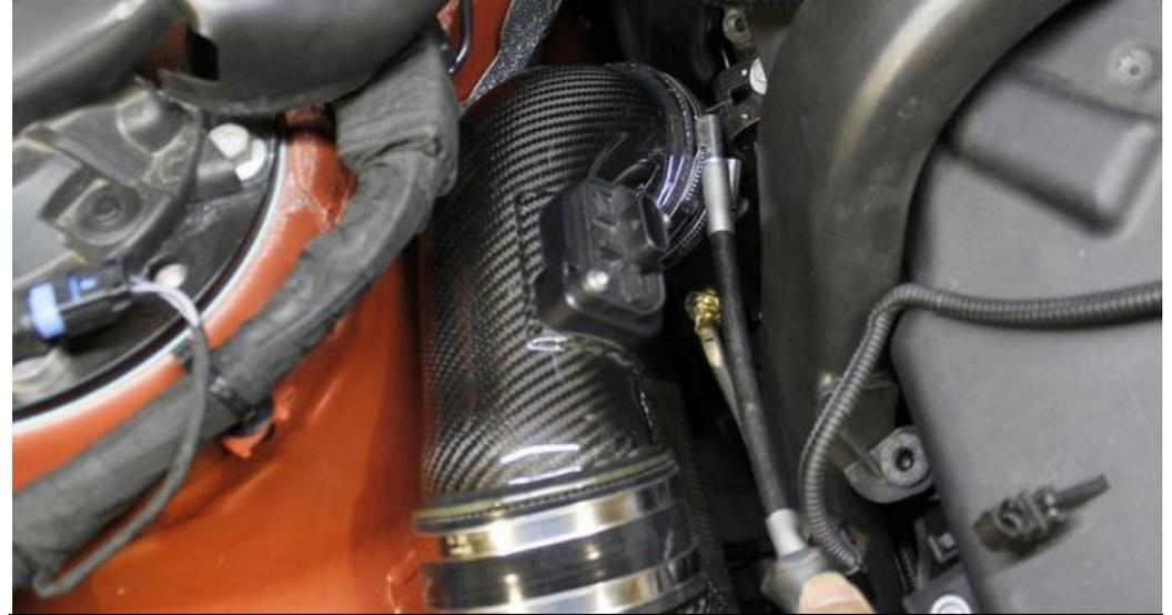
35. Now tighten the lower clamp on the tube – ensure there is no gap between the flange on the carbon tube and the silicon.
