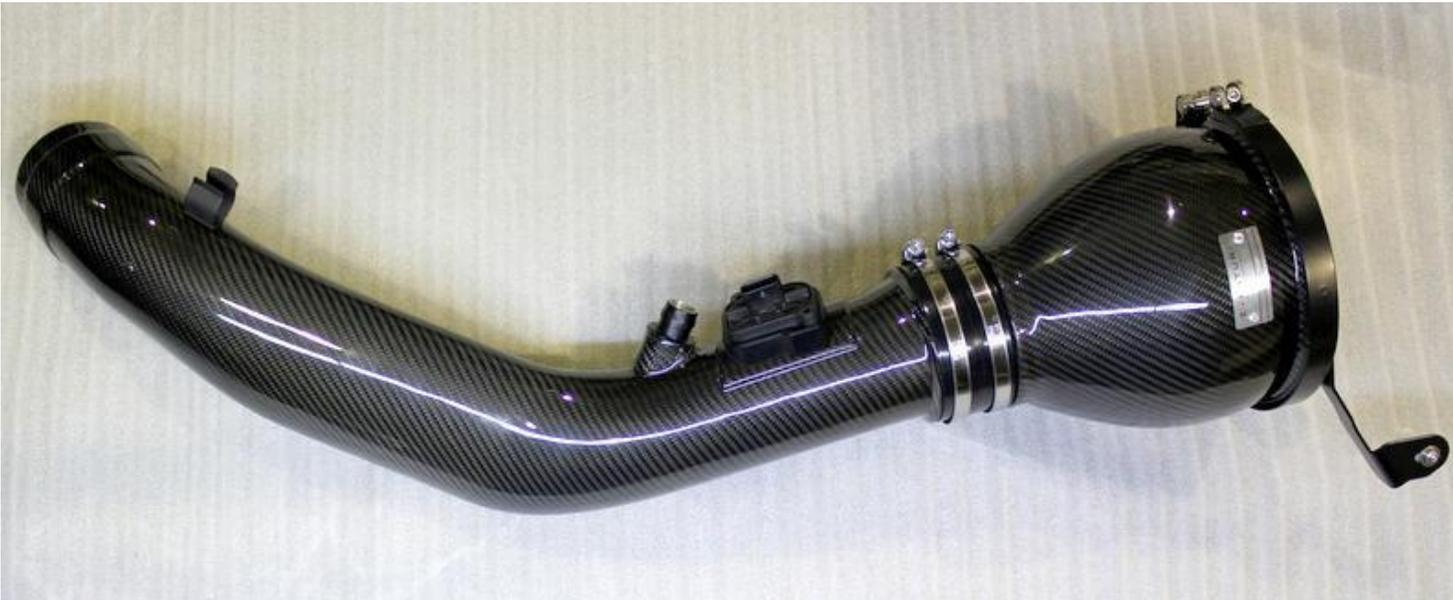
37. Assemble the right side intake with the long carbon tube as shown using the remaining silicon coupler and hose clamps. When pushing the silicon coupler onto the housing **DO NOT PUSH ON THE FILTER ITSELF**. Tighten the clamp on the housing, leave the clamp on the tube loose to allow it to rotate.
