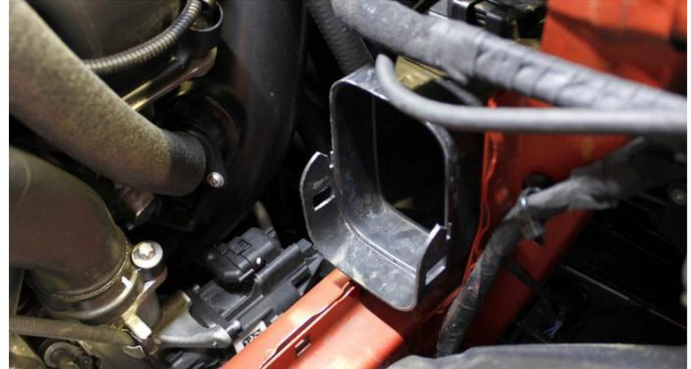
25. Looking at the other side – identify the 2 holes on the stock opening which will again be used for location and securing the left side duct.
