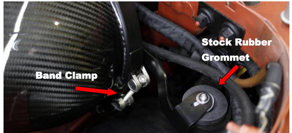
35. Push the plastic boss on the mounting bracket into the stock rubber grommet fully. You might need to rotate the Band Clamp to avoid the duct. This has been left loose to allow rotation.
