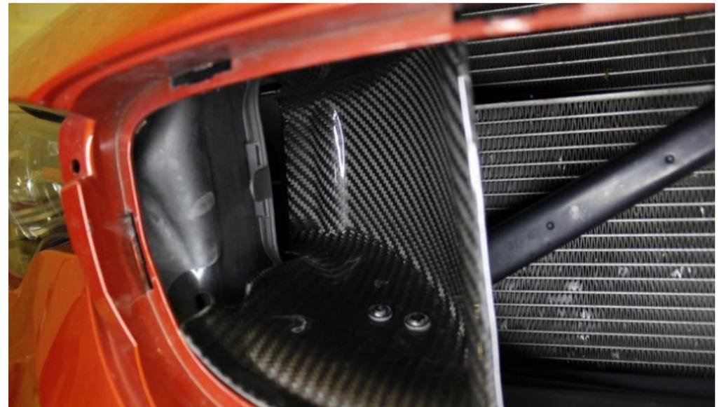
53. The back of the scoop should be sitting inside the stock duct opening as shown.
