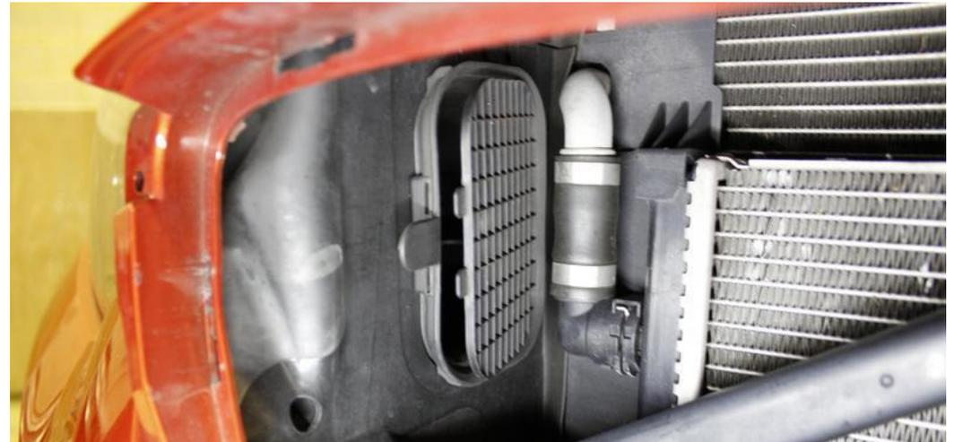
49. Here you can see the front of the grid has been released and can now be removed. Do the same for the other side.
