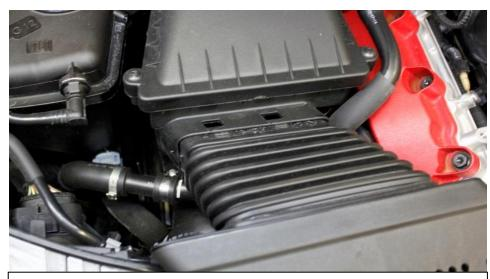
4. Pull the corrugated duct feeds out of the airboxes. Push the fronts down to release the tabs holding them into the airboxes on both sides. Once removed from the airboxes, remove the ducts completely.
