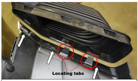
17. Finally, remove the feed from the base by levering it off the remaining 3 tabs shown with white arrows. In some instances there may be some adhesive holding a corner in place. Use the screwdriver to free it. The plastic used on these parts is very brittle so there is a chance some locating tabs may break. Although these are not essential – try to be as careful as possible.
