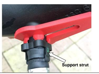
3. Push the tool onto the breather inlet – it will snap into place. Make sure it is positioned with the support strut of the breather facing the back/front of the tool as shown.
