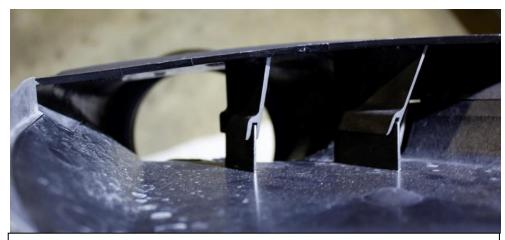
39. Line up the vertical tabs on the cover to the lower duct as shown.
