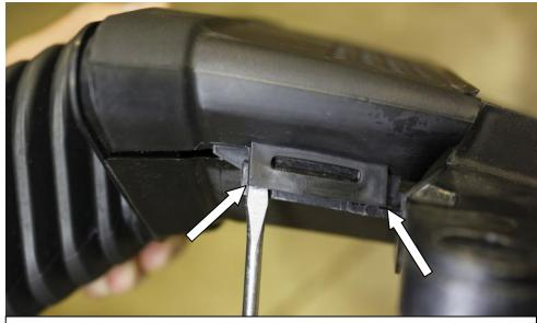
14. Using a flat head screwdriver, carefully prise open the tab on one side of the cover from the 2 edges. These tabs are easily broken so take your time doing this.
