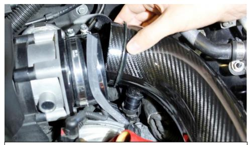
56. Line up the RHS carbon tube with the breather connector and angle it in while pushing the tube into the silicon. Make sure the hose clamp around the silicon is sufficiently loose.
