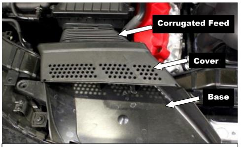
13. Now we need to separate the duct which was previously removed, into 3 pieces. The base, cover and corrugated feed.
