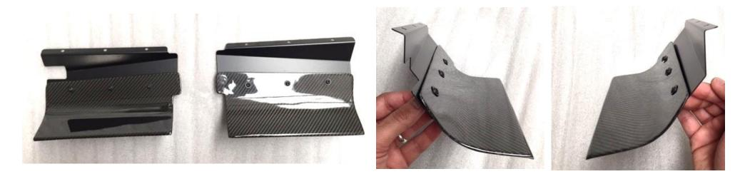
20. Take 6 black flanged bolts and lock nuts and fasten the scoops to the plates as shown. The holes in the scoops should line up with the slots on the plates.
