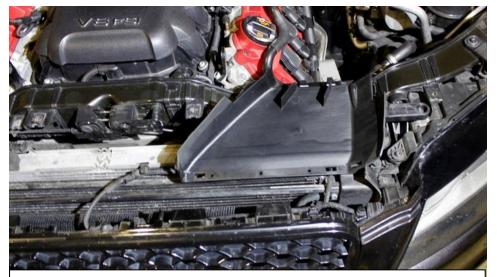
21. Take the right side duct and secure it into position with the 2 screws previously used.
