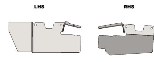
30. Identify the LHS and RHS heat shields as shown.
