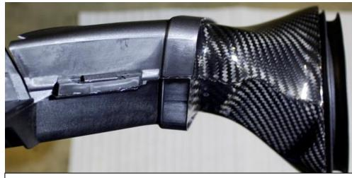
41. Other side locked into place. If these side tabs are completely broken and cannot hold the top and bottom duct parts in place – then you can use 4 flanged bolts and nuts to secure the carbon duct to the plastic duct.
