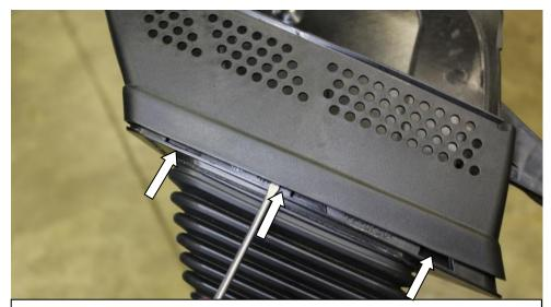
16. Using small flat head screwdriver, slide it between the cover and the corrugated feed. Lever the screwdriver upwards carefully to free the cover from the remaining tabs holding it to the feed. Remove the cover completely.
