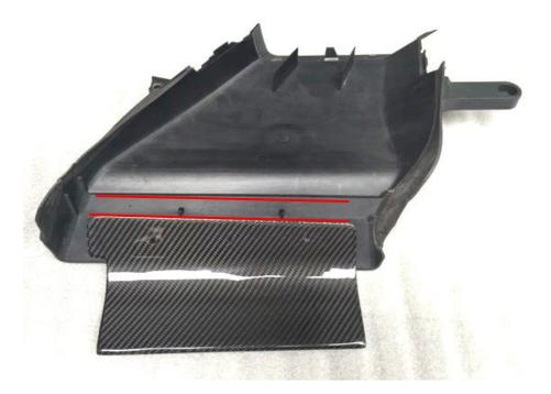
28. Secure the stock duct in place with the 2 screws removed previously. Lower the scoop into place and line it up with the edge highlighted above. Ensure the scoop sits flat against the inside of the grill and mark the 3 holes through the scoop onto the duct.
