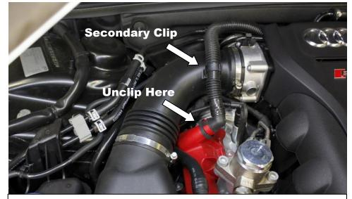
6. Unclip the crank vent hose from the valve cover by squeezing in the 2 sides to release the clips. Pull this off the valve cover and then out of the secondary clip on the inlet tube. Move the hose away for more clearance.
