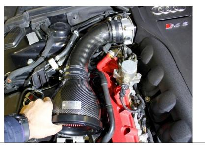
45. Take the LHS Housing and push the silicon on the back of the housing into the carbon tube. Lower the tube and housing onto the heat shield.
