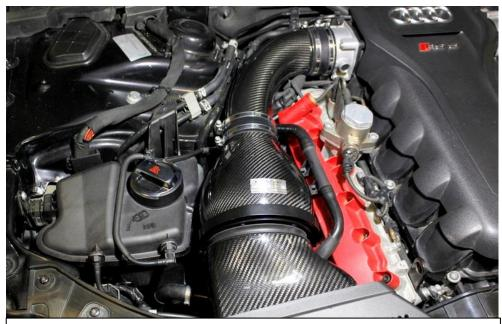
52. Tighten the remaining hose clamp around the carbon tube and place the duct back into place. Do not overtighten the clamps. Secure the stock duct with the 2 screws previously removed.
