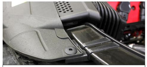
2. The plastic rivets can be removed by firstly pushing in the centre tab and then prying the main body upwards. Careful not to press the centres all the way through as they will drop into the engine bay. Once all fasteners are removed – pull the duct cover off.
