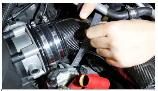
57. Now with the breather positioned into the tube connector – grab the Velcro straps on either side and pull upwards to click the breather into place.
