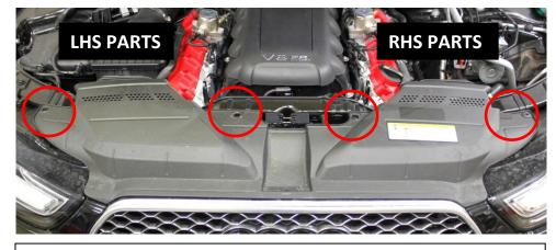
1. Remove the 4 Plastic Rivets as circled (or torx screws for earlier models) securing the duct cover in place. We will refer to the left hand side and right hand side parts as indicated above.
