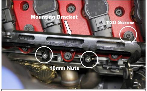
10. Remove the airbox mounting bracket by removing the 2 x 10mm nuts and 1 x T20 Torx as shown above. You don't need to remove the other T20 Torx screw. Once the bracket is out – refit the T20 screw,
