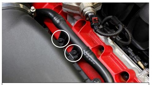
7. Remove the 2 x T30 Torx screws holding the air pipe in place on the airbox.
