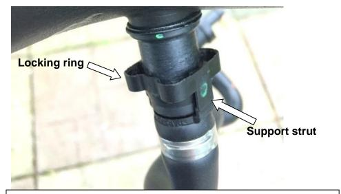
2. The later type breather vent hoses are locked in place by 4 tabs. We will use our supplied tool to remove this hose. The locking ring is supported by 2 plastic struts – we will insert our tool facing one of these struts.
