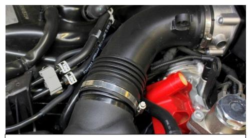
8. Loosen the hose clamp between the inlet hose and the airbox. Push the inlet hose off the airbox.
