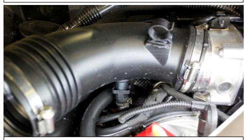
11. Loosen hose clamp around the inlet tube and throttle body. Pull the tube out of the throttle body to give you more room to access the breather hose underneath.
