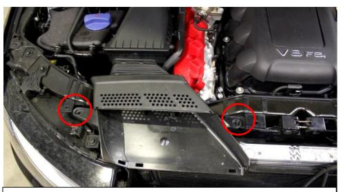
3. Remove the 2 x T25 Torx screws holding the LHS and RHS ducts in place. Keep these screws safe as they will be required for refitting the duct later.
