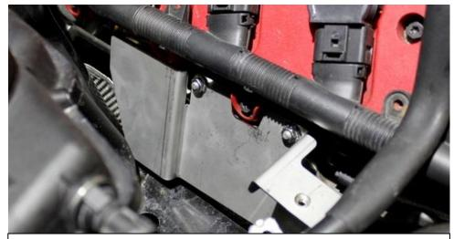
31. Take the LHS heat shield and mount it onto the 2 studs previously used for the stock airbox bracket. (See step 10). Secure into place with the 2 provided 10mm nuts. Heat shield shown in silver for illustration purposes.
