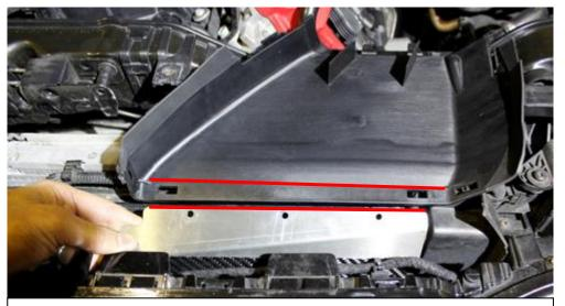
22. Take the RHS Scoop and Plate assembly, place it behind the grill and line up the edge of the metal scoop plate with the stock duct as highlighted here in red.
