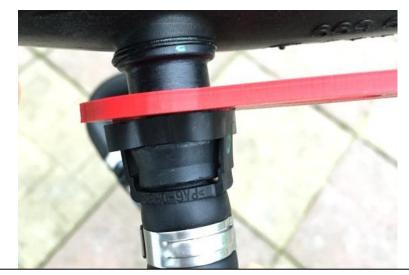
4. Push the tool down so that the 4 extrusions go into the 4 openings of the locking ring fully.
