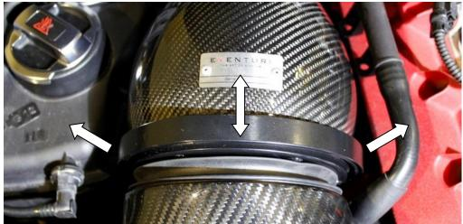
50. Adjust the housing by pivoting left and right, also can be moved back and forth to ensure a good seal. The seal should be touching the housing – not pressed up tightly against it. Once adjusted, make sure the bracket is still lined up with the M6 clinch nut on the heat shield. You can rotate the housing to line it up.
