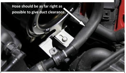
51. Remove the duct and secure the bracket using one of the supplied M6 Bolts and lock washers. Also secure the secondary air hose to the bracket with another nut and washer. This air hose MUST be as far towards the engine as possible to give the carbon duct clearance – move the clamp along the hose if required to line up with the bracket.
