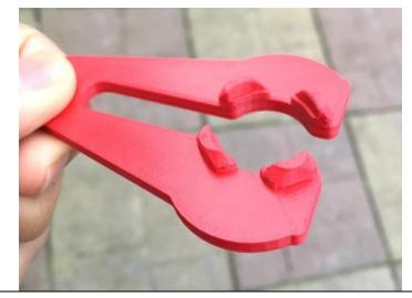
2. The 3D printed tool (colour may vary) has 4 tapered extrusions. Each of these pushes out the locking ring of the breather hose and releases the tabs holding it onto the inlet tube.
