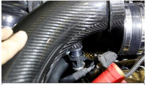
43. Take the LHS tube and push the breather tube back into the fitting at the bottom of the tube. It will click into place.
