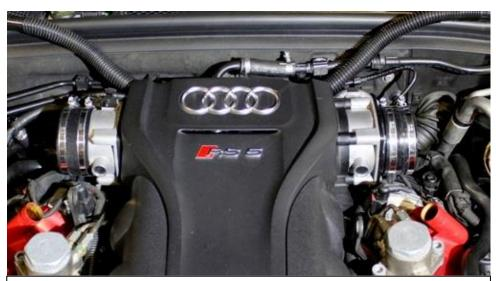
33. Take 2 of the silicon couplers and install onto the throttle bodies. Push them on fully and tighten the clamp over the throttle body. Leave the other clamp loose.
