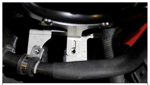
46. The bracket on the housing should sit on the heat shield. The clamp on the secondary air hose should sit on top of the bracket.
