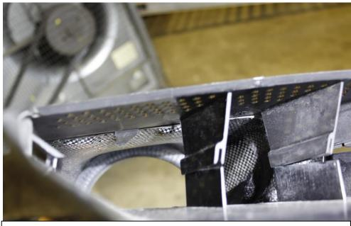
38. Take the top cover for the LHS stock duct and push it into the carbon duct – the next photo shows how the cover should sit on the carbon.
