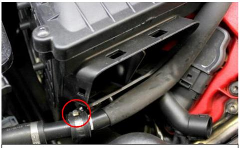
5. Starting with the left hand side (as you look at the engine) remove the 10mm nut holding the secondary air pipe in place. Lift the pipe clamp up and away from the airbox.
