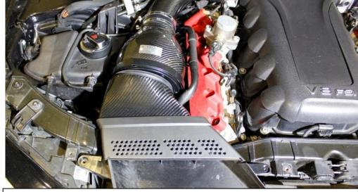
48. Take the LHS duct assembly and put it into place – the scoop goes in first then lower the duct and move it forward towards the housing. Line up the securing holes on the sides of the stock duct – do not secure yet.
