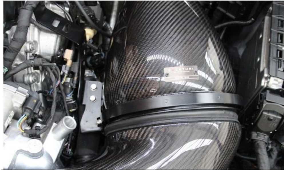
54. Line up the filter housing with the duct and then use the Nylock Nuts to secure the 2 screws on the bracket.
