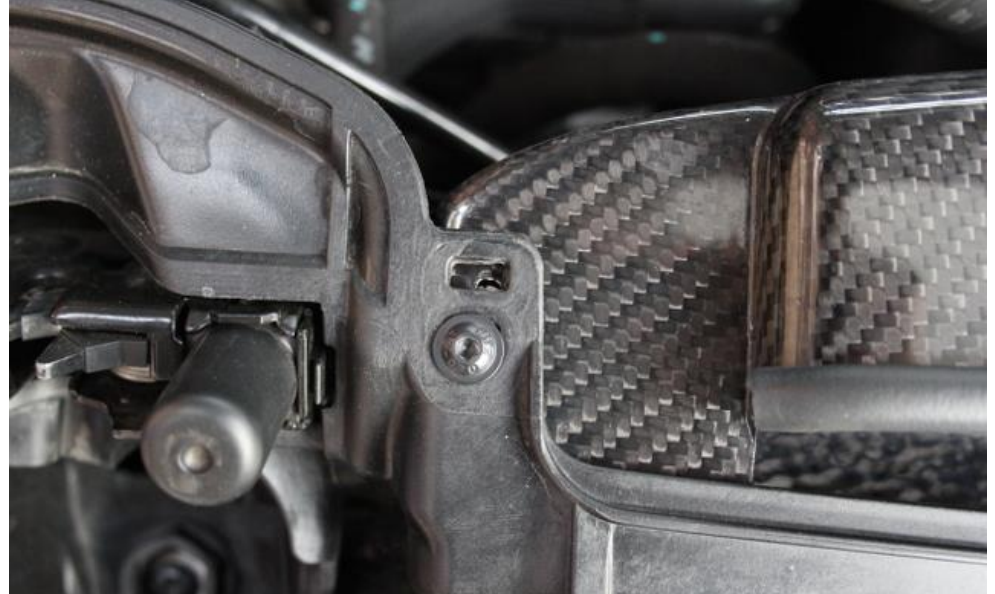
50. – line up the hole on the panel with the correct hole on the duct as shown in previous step. For RS3 Secure with a supplied M5 Screw. For TTRS secure with the original stock screws.
