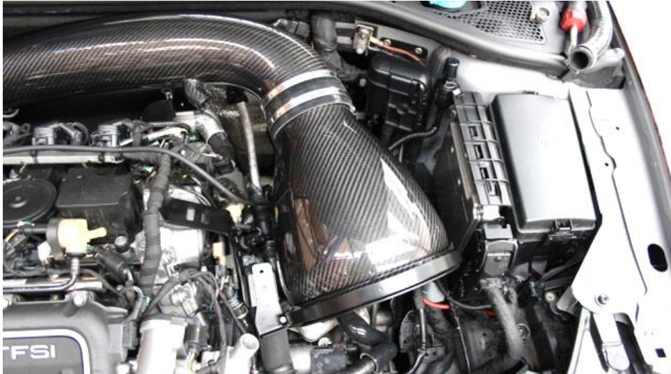
41. Push the filter housing into the silicon coupler on the tube as shown. Eventuri plaque should be facing upwards and the bracket should rest on the previously mounted bracket.
