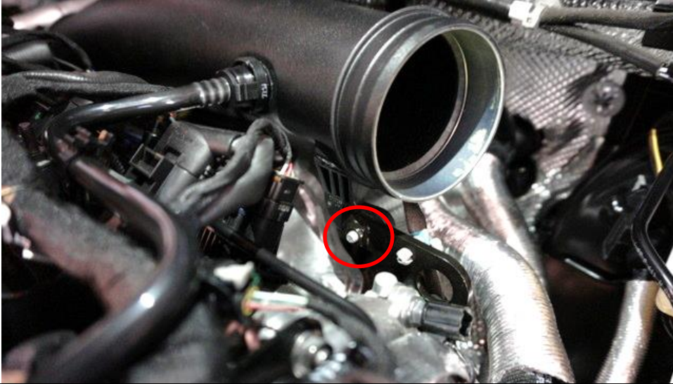
9. Remove the screw securing the Turbo Tube.
