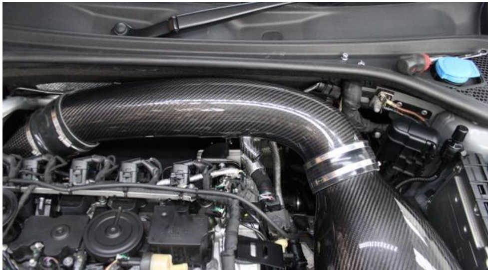
55. Pull the carbon tube into the filter housing, rotate if required for clearance over the brake fluid reservoir and secure the remaining hose clamps. Do not use a ratchet to tighten it – it just needs to be finger tight. Over tightening can damage the tube.
