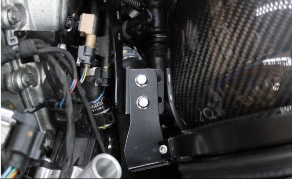
53. Align the holes on the filter bracket with the slots on the engine bracket and push the 2 screws through – it may be easier to push the screws upwards from underneath so that the access is easier for the nuts.
