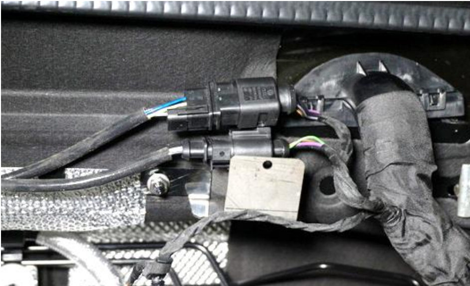
17. Install the new bracket onto the threaded stud as shown and secure with the supplied M6 Nut.
