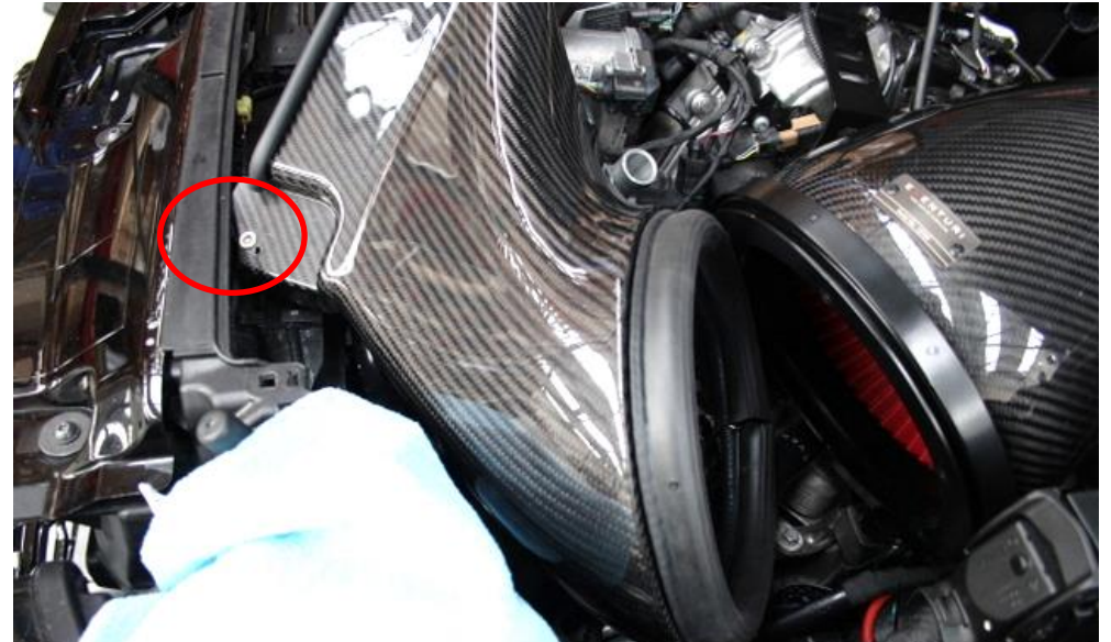
46. Another angle of the duct angled into place – notice the rear edge is inside the slam panel.
