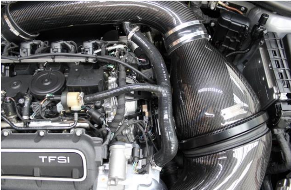
57. Install the breather hose as shown for the 2 variants and secure the hose clamps.
