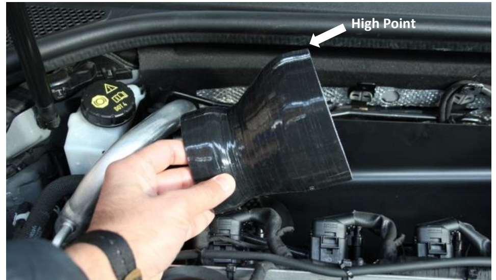
32. Place the reducer onto the stock turbo inlet tube with the appropriate hose clamps and the high point facing upwards as shown.
