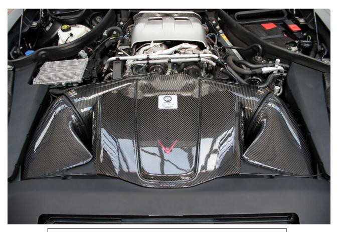
40. Fit the new engine cover - you can remove the Engine Builder Plaque from the original cover and fit it to the new one.
