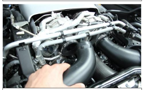
8. Loosen and remove the tube to the Turbo inlet.
