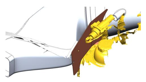
37. Install the LHS shield to the LHS of the front trim panel using the OEM push clips. CAD image show for clarity.
