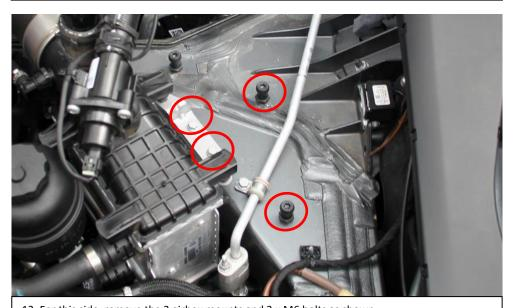
12. For this side, remove the 2 airbox mounts and 2 x M6 bolts as shown.
