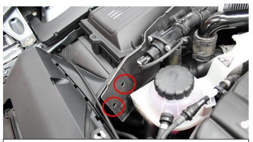
1. We will start by removing the left side stock airbox. Remove the plastic centre cover. Remove the 2 plastic push clips in the heat shield.
