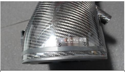
22. Take the LHS Housing and pull the black band back as shown – otherwise it will get caught on the duct during installation and come off.
