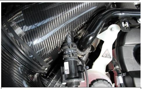
26. Push the silicon tube onto the housing and secure with the clamp.
