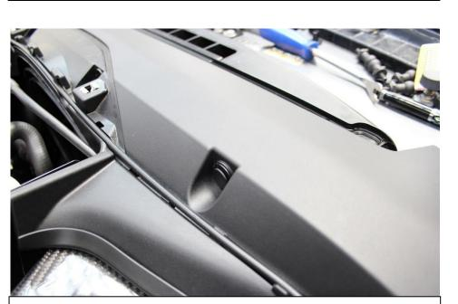
39. Push the bonnet cable back into place and secured the panel with the OEM push clips.
