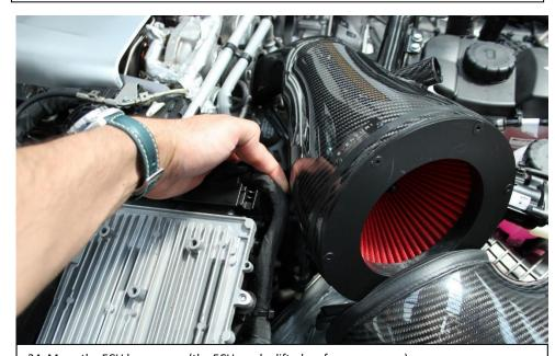
$24. \ \mbox{Move the ECU loom away}$  (the ECU can be lifted up for more space).
