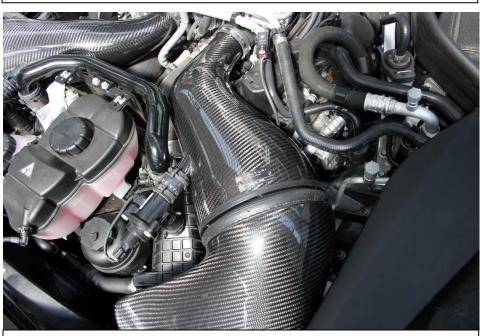
31. Line up the housing with the duct and secure the silicon breather hose as with the LHS Housing. Secure the hose clamp at the turbo side. Do not over tighten.
