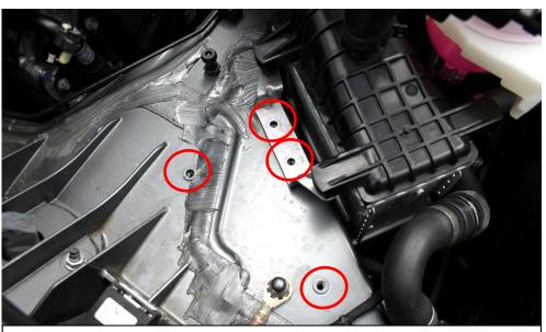
10. Remove the 2 Airbox Mounts and 2 x M6 bolts shown.
