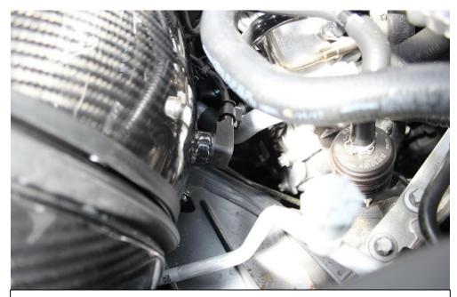
32. Connect the MAP sensor plug to the housing.
