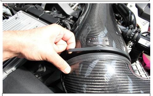
28. Move the band back into place so that it covers the join between the filter and the carbon housing.
