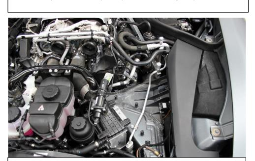
11. Repeat the process for the right side and remove the airbox assembly.
