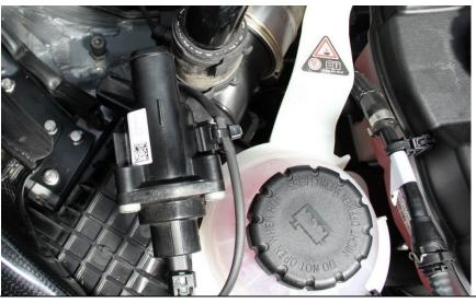
6. Remove the rubber hose completely and retain the spring clamps.
