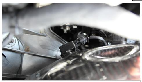
29. Reconnect the MAP senor plug – it will click into place. Lock the plug with the small tab at the top.
