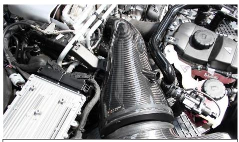
25. Rotate the housing into place. There is a recess on the housing for the strut brace and also for the ECU loom. Rotate the housing to line up these recesses.
