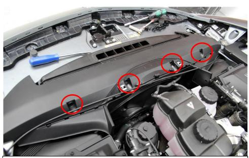
3. Remove the  $4 \times 10^{-2}$  x plastic push clips and unclip the bonnet cable over the front plastic trim panel.
