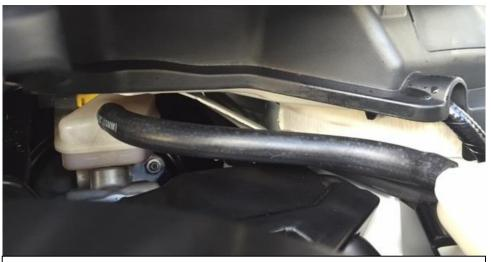
16. Push the new brake hose onto the brake cylinder fully and secure with the original spring clamp. Then push the other side into the brake reservoir and secure with remaining spring clamp. We will now install the cold air duct and intake housing assembly before completing the relocation procedure.
