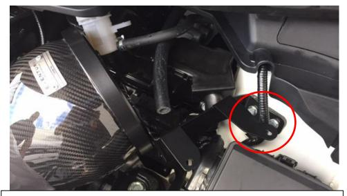
36. Now secure the intake using the 2 supplied M6 bolts. Duct and brake fluid reservoir not shown for illustration purposes.
