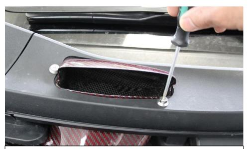
27. Position the duct to line up the threaded inserts with the holes on the panel and secure with the supplied screws. Do not over tighten them. Location of the holes may vary depending on LHD or RHD version.
