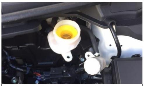
12. Empty the brake fluid reservoir using a pump or simply pouring into a container. Wipe away any spillage in the engine bay.
