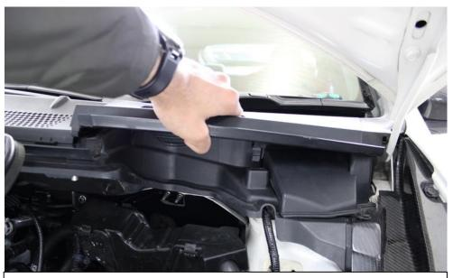
18. Pull the plastic panel upwards to unclip it.
