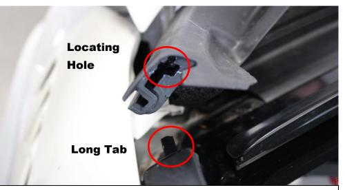
20. Now pull the panel down to unclip from the windscreen panel. There is a long tab which locates into the hole in the panel as shown. Remove panel completely
