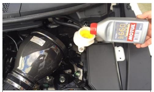
40. Fill the brake fluid reservoir with DOT 4 fluid. Do this slowly to allow the fluid to flow down the new hose. Continue to top up until fluid settles at the top of the yellow chamber. Secure the cap back onto the reservoir.
