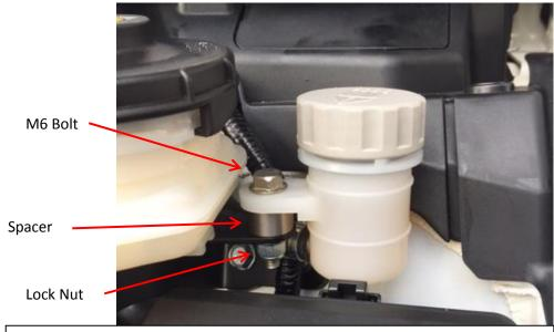
38. Using the thinner spacer – secure the clutch fluid reservoir to the housing bracket as shown.
