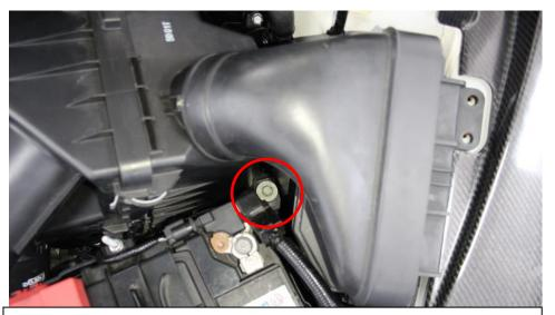
5. The Airbox is held in with 2 10mm bolts. Remove the front one as shown behind the battery.
