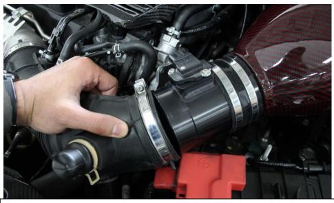
34. Push the stock rubber hose onto the MAF tube – make sure the clamp is loose. Support the housing while pushing the hose on.
