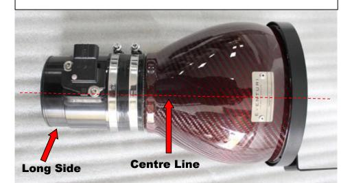
31. Assemble the tube to the carbon filter housing with the supplied silicon hose as shown. The short side of the MAF tube should be inserted into the silicon. This leaves the long side exposed. The sensor should also be oriented slightly off-centre as shown here and in the next step.
