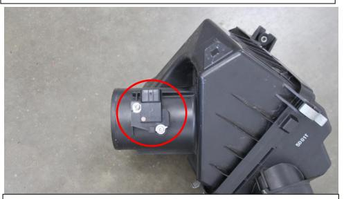
7. Remove the MAF sensor by unscrewing the 2 screws holding it to the airbox.
