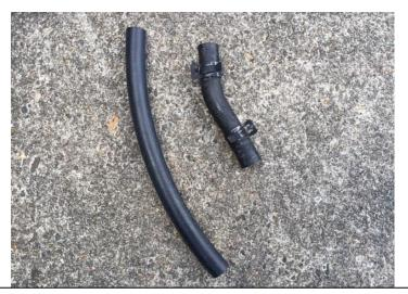
15. Remove the hose completely. Now transfer the spring clamps to the new longer brake hose supplied.
