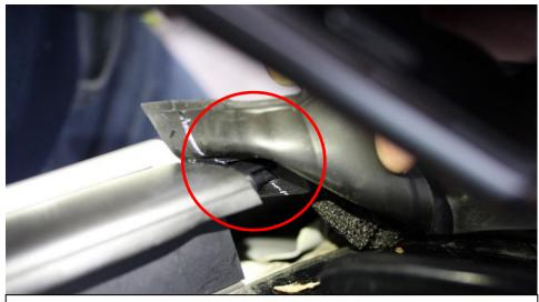
24. Now push the locating tab from the windscreen panel into the hole of this new panel as shown.
