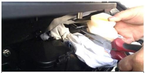
13. Compress the spring clamp around the brake hose and push further down the hose to allow the reservoir to be removed.
