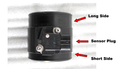
30. Install the MAF sensor onto the supplied sensor tube as shown with correct orientation. Secure with the two supplied M4 screws.
