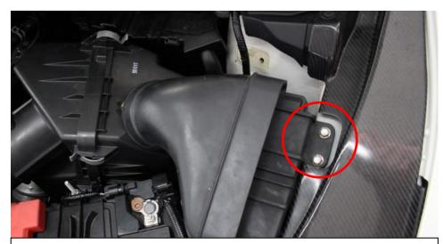
4. Remove the 2 10mm bolts from the intake duct.
