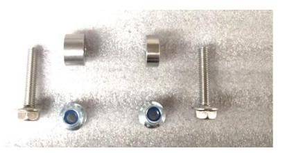
37. identify the 2 spacers, lock nuts and bolts which will now be used for the reservoir relocation. The thicker spacer will be used for the brake fluid reservoir.
