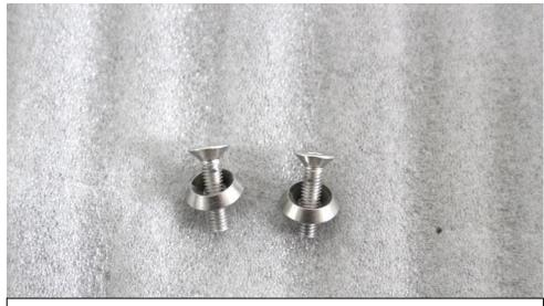
26. We will use the supplied countersunk screws and washers to secure the duct to the plastic panel.
