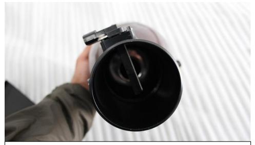
32. Orientation of the MAF sensor with the metal badge on the housing facing upwards.
