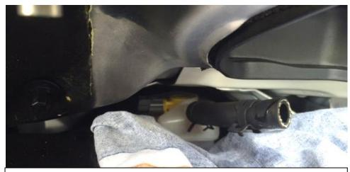
14. Place a cloth under the assembly to catch any fluid and carefully remove the reservoir from the hose. Now compress the other clamp near the cylinder and pull it away to allow removal of the brake hose.
