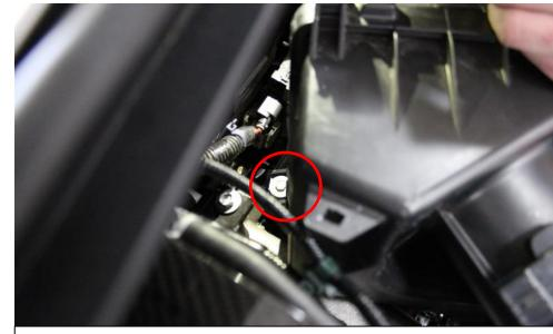
6. Remove the remaining bolt which is located at the back of the airbox. Now pull the entire airbox assembly out.
