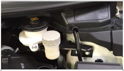
8. Now we will relocate the brake and clutch fluid reservoirs.
