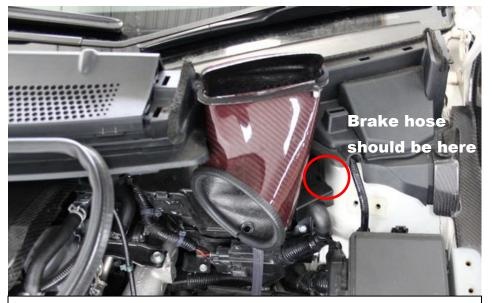
21. Place the carbon duct into the space revealed under the removed plastic cover. This will be secured in the coming steps. Ensure the extended brake hose is routed around the side of the duct. Hose not shown in the photo.
