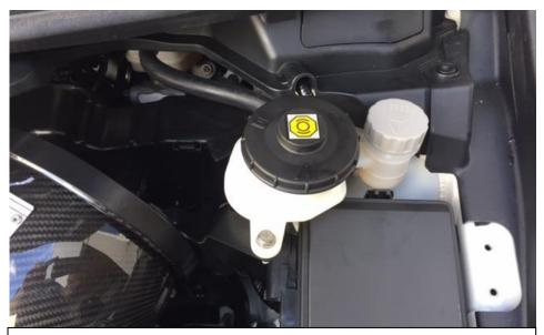
39. Use the remaining thicker spacer for the brake fluid reservoir and secure to the housing bracket in the same way.
