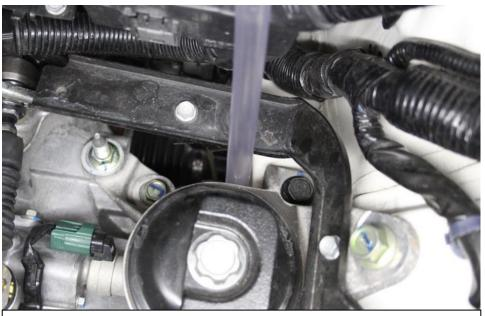
22. Position the drain tube as shown.
