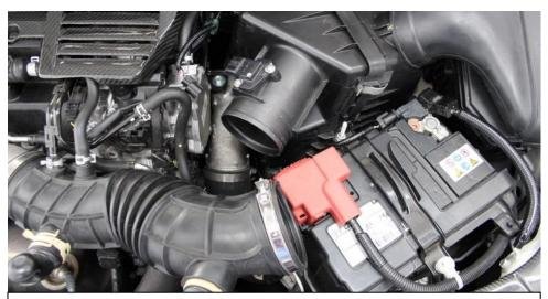
3. Loosen and remove the rubber intake hose from the airbox.
