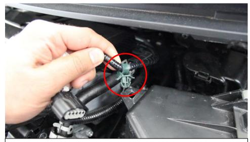
2. Remove the sensor wiring harness from the airbox – push the green tabs inwards to allow you to pull the clip out. Unplug the MAF Sensor plug.
