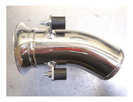
12. Bolt on cotton reel rubber mounts with two M6 nuts and washers to inlet pipe.
