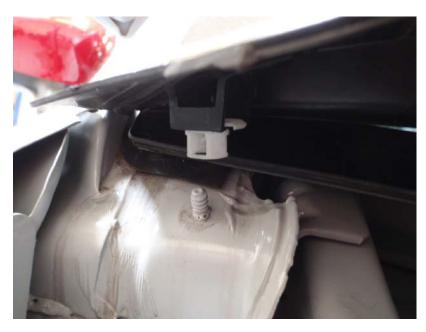
8. Now lift the panel upwards and in the far corners you will see a white clip. Pull upwards to remove.
