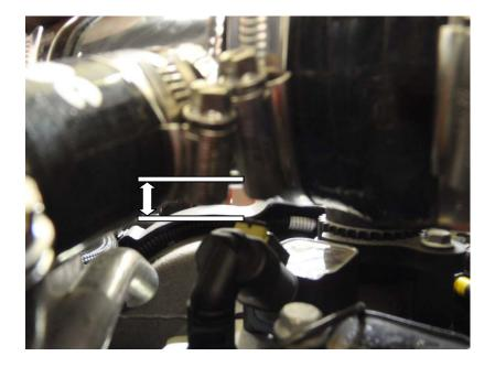
16. Tighten all the jubilee clips in such a way that there is a gap of at least 5mm between the coil pack and the bottom of the pipe. The installation of your induction kit is now complete!
