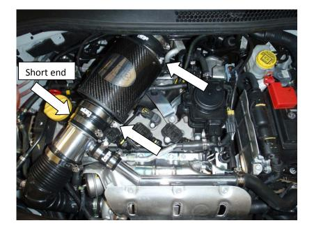
15. Put the silicon hoses on the filter with the 90 diameter jubilee clips, and tighten. Place all the parts of the induction kit loosely in position make sure the aluminum pipe indicated above has the short end facing towards the back of the engine.
