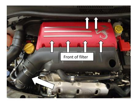
4. Pull the plastic pipe off and pull the filter box upwards with an even pressure at the front until it has came away from its rubber mounts. Then pull upwards with an even pressure the back of the filter where indicated to release from the rubber mount at the back.
