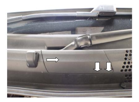
5. Remove the scuttle panel, by first removing the wiper blade covers by holding the right side and pulling towards the front of the car. Then pull from the left to the right to completely remove.
