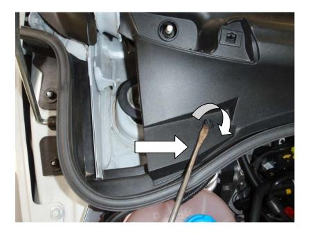
7. There are three small plastic clips holding the front of the cowl. Rotated by 45 degrees they will lift up slightly. Place the screw driver in the gap and pull up the rest of the way to pull the clips out.
