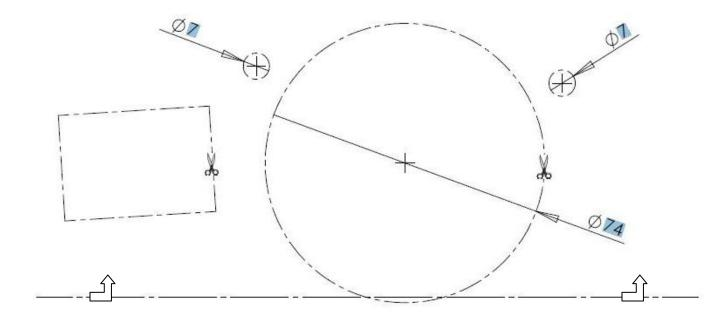
Above is the template for cutting the hole in the scuttle panel. Cut out the square and fold up the bottom line. If you are using a hole saw, mark through the center of the 74 diameter hole if you are using a jig saw, cut out this hole for positioning. Please see step 12.
