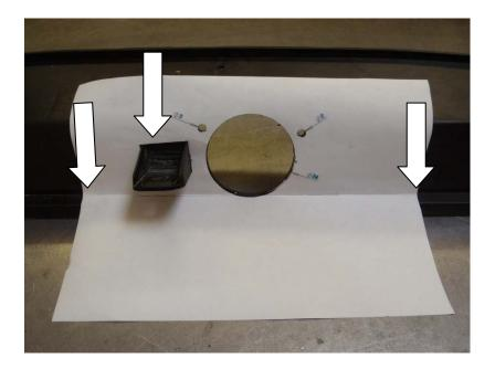
11. Place the scuttle panel on a table with the rear facing towards you. You will see a bracket just off the center line of the panel. Cut out the paper template according to which tools you have and fold on dotted line. Match up the folded line with inside edge, and place over the bracket mark the holes through the template then drill and cut the holes out.
