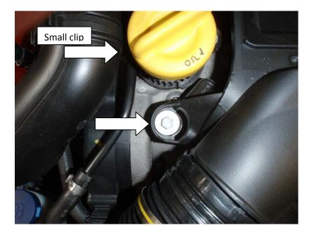
3. Remove a small clip under the intake and undo the 10mm bolt holding the filter.
