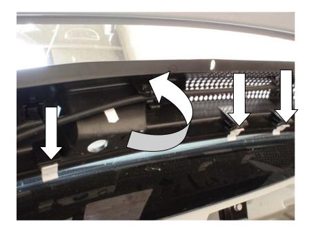
9. Gently rotate the panel upwards releasing the 6 white clips from under the windscreen.
