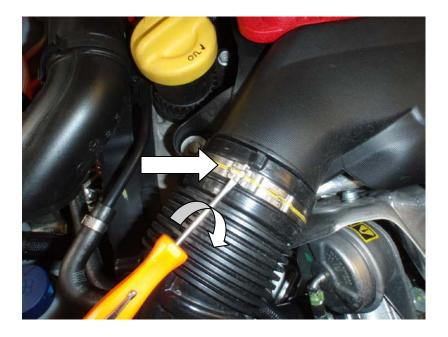
1. Park the vehicle securely, Open bonnet and start with removal of original filter. You will need to break off the 'use once' only clips by placing screwdriver between the raised section of clip and twisting the screwdriver around.
