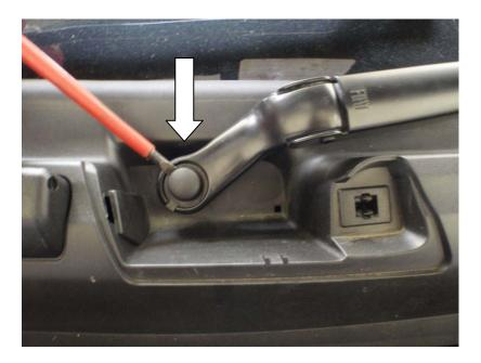
6. Using a screw driver, carefully pry off the small covers hiding the nuts that hold the wipers on. Avoiding marking the paint. Undo the 13mm nuts and pull off the wipers keeping a note of their position.
