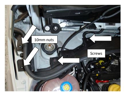
10. Undo the five pozidriv / Phillips screws and undo the four plastic 10mm, nuts and remove the plastic scuttle panel.
