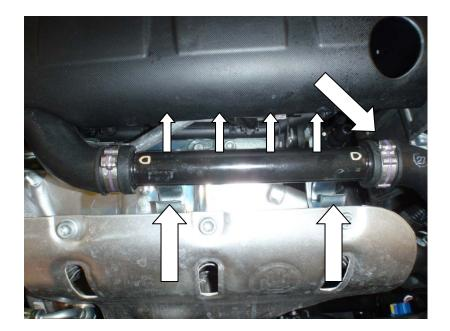
2. Repeat to break the use 'once clip' on the right of the photo and pull the metal pipe up out of the clips.
