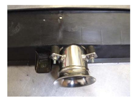
13. Bolt the inlet pipe to the scuttle panel with two M6 bolts and washers.
