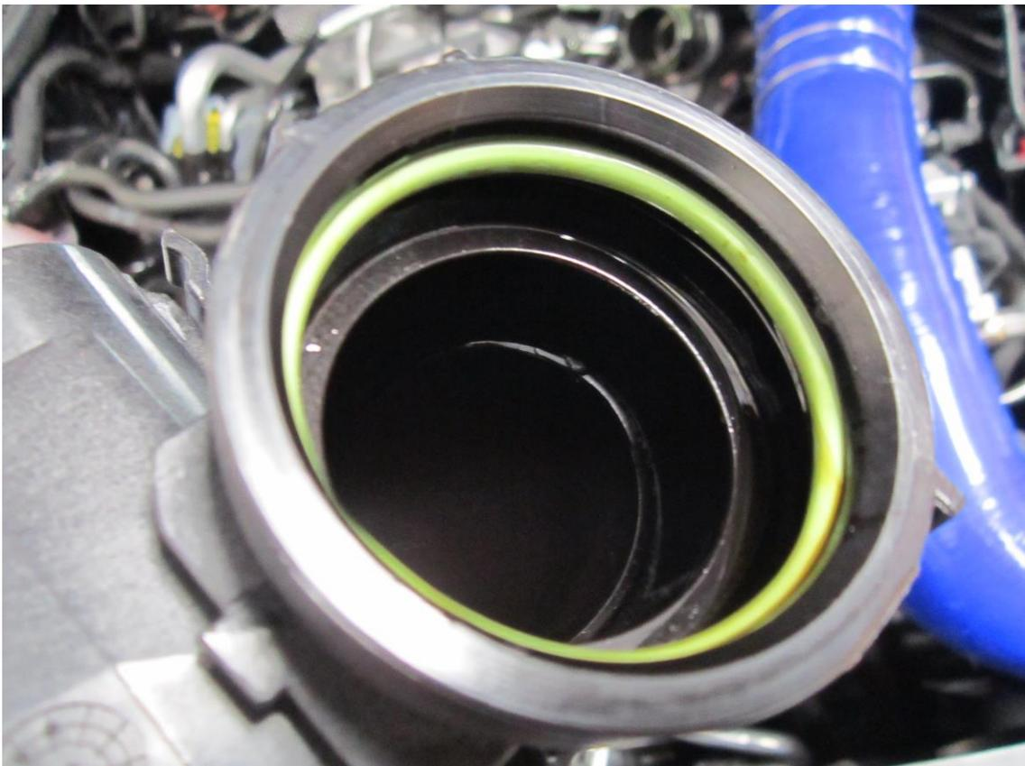
7. Place both the Forge Motorsport billet couplers into position and push into situ until you hear a positive click.
