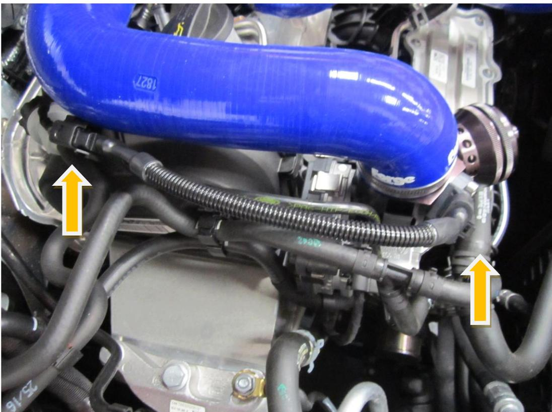
12. Remove the 2<sup>nd</sup> map sensor from the inlet manifold.
