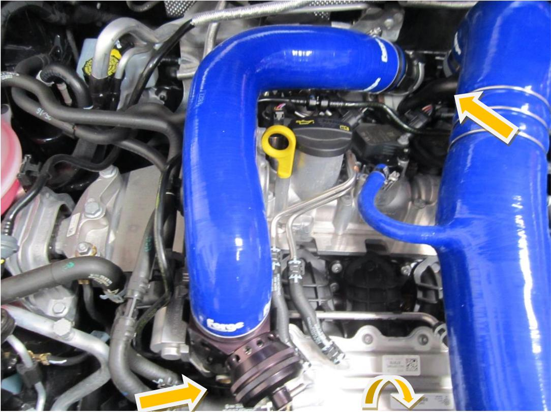
9. Remove the map sensor from the OEM boost pipe by prying the clips outwards and pulling the map sensor away from the housing.
