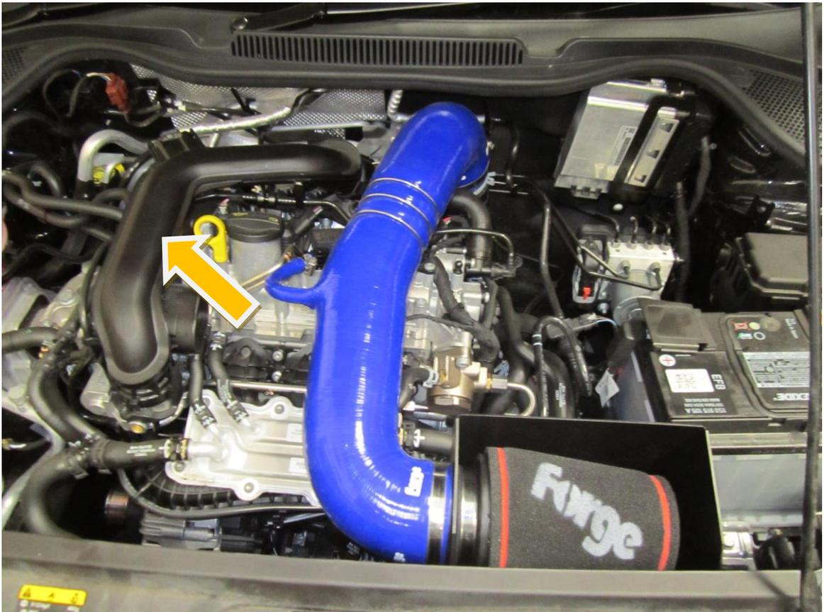
2. Unplug the wiring loom from the map sensor housed in the boost pipe.
