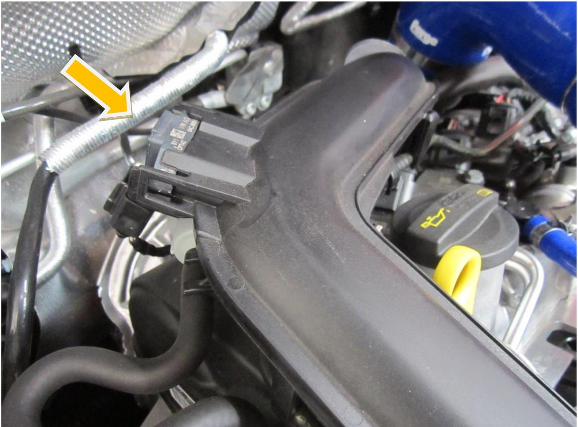
3. Unclip the vacuum hose from the side of the boost pipe.
