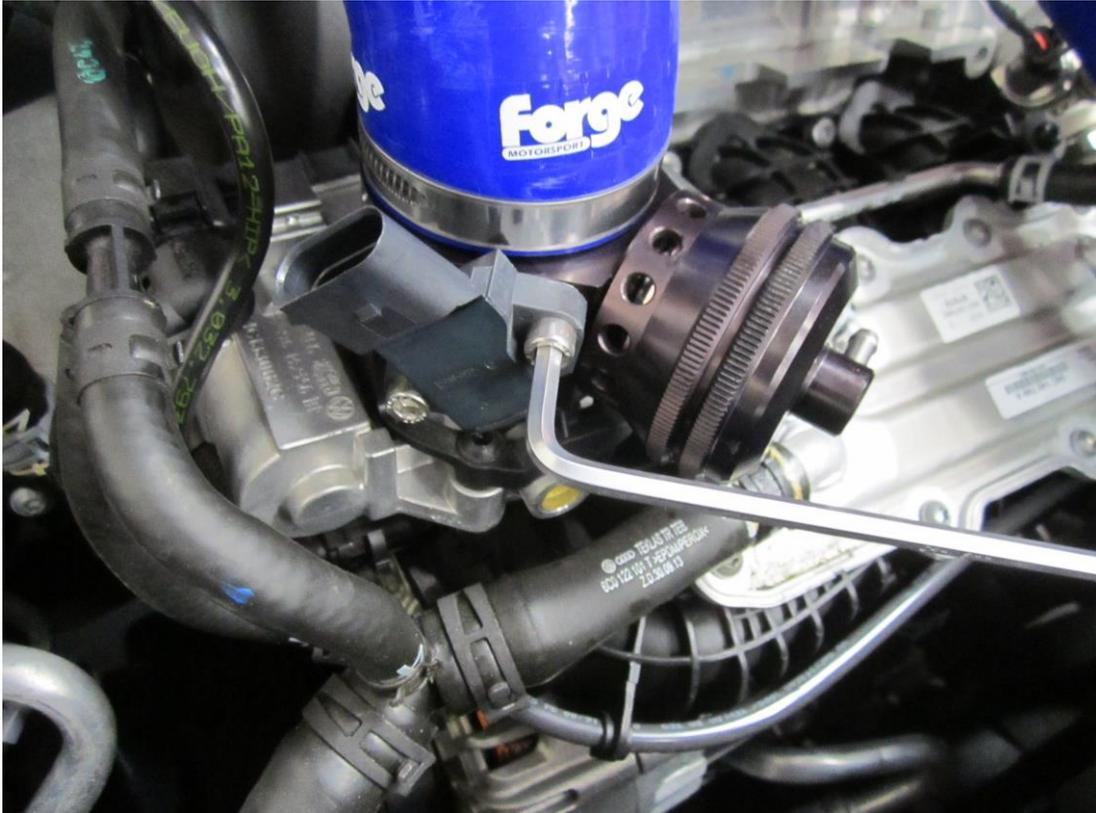
11. Plug in the wiring loom extension between the map sensor and the OEM wiring loom.
