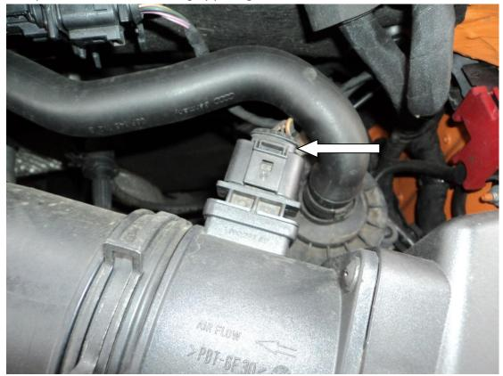
5. Remove the noise generator pipe running along the side of the air box by unclipping the 2 clips.
