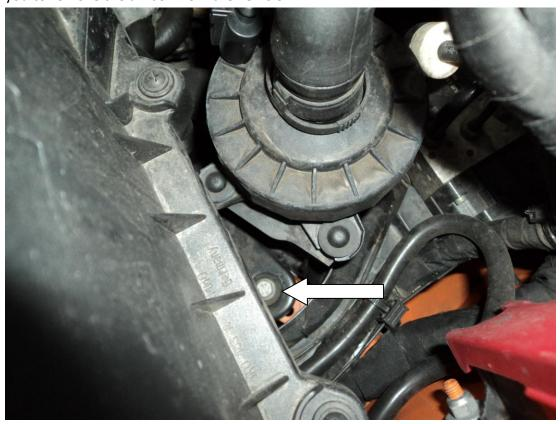
8. You will now need to undo the 10mm bolt holding the air box bracket to the vehicle using a 10mm socket and matching ratchet.
