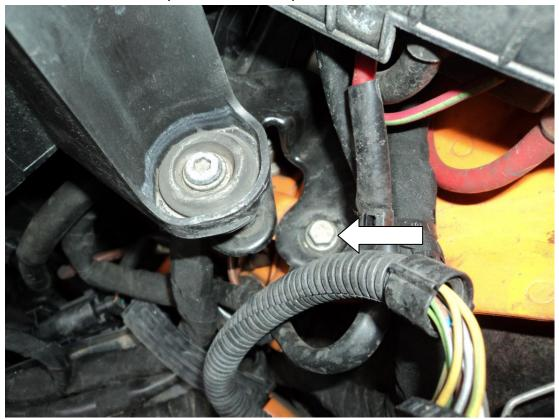
7. Using a 10mm socket and matching ratchet, undo and remove the 10mm bolt situated at the rear of the air box next to the noise generator. This will now allow you to remove the air box from the vehicle.
