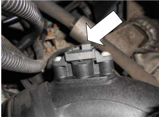
13. With a firm pull release the coupler from the throttle body and remove the pipe from the vehicle.
