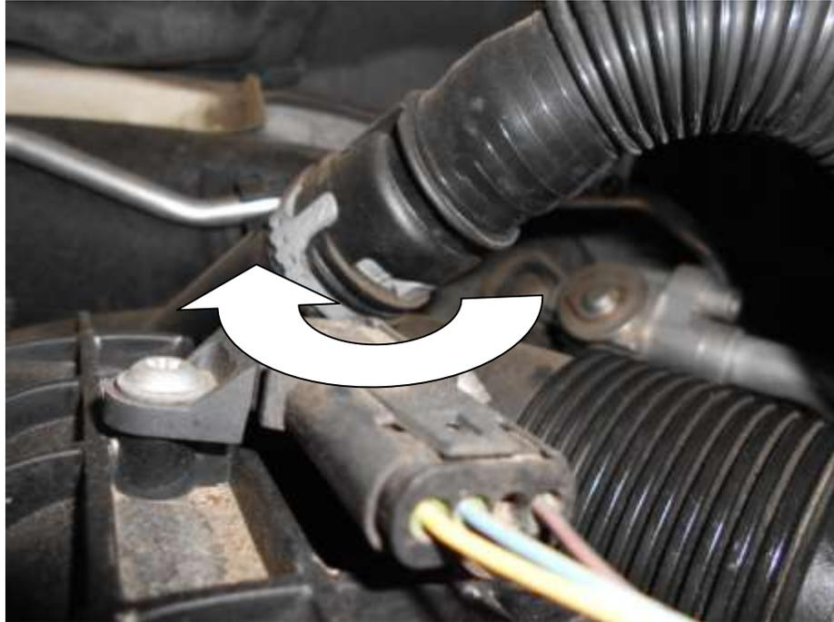
9. Using a flat blade or 7mm hose clamp driver screwdriver undo the jubilee clip.
