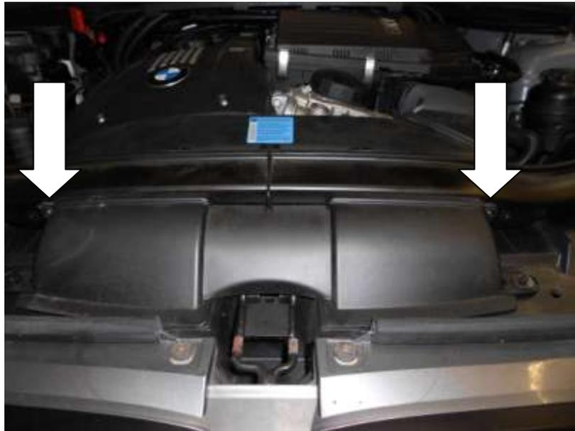
2. Unclip the ducting from the front of the air box and remove the duct.
