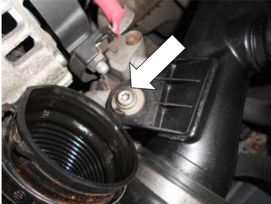
11. Using a flat blade screwdriver or pliers remove the spring clip from the throttle body hard pipe.
