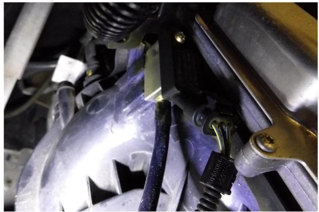
8. Attach the vacuum tube to the nipple of the vacuum take off block and using the m5 x 35mm screw provided tighten in position.
