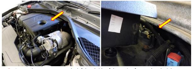
5. Locate the map sensor on the left hand side of the engine fastened to the inlet manifold beneath the side of the ECU.
