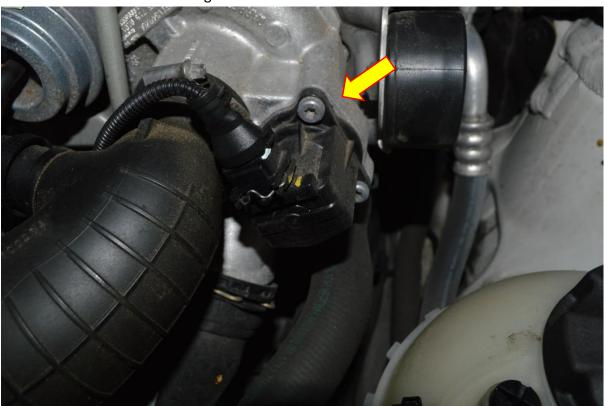
3. Place the O-rings provided into the Forge Motorsport valve before installing into position on the turbo.
