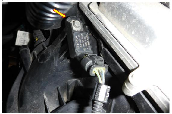
7. Remove the map sensor and place the vacuum take off block in its position with the map sensor placed into the forge take off block, the ecu tray may need lifting slightly to fit both parts into situ.
