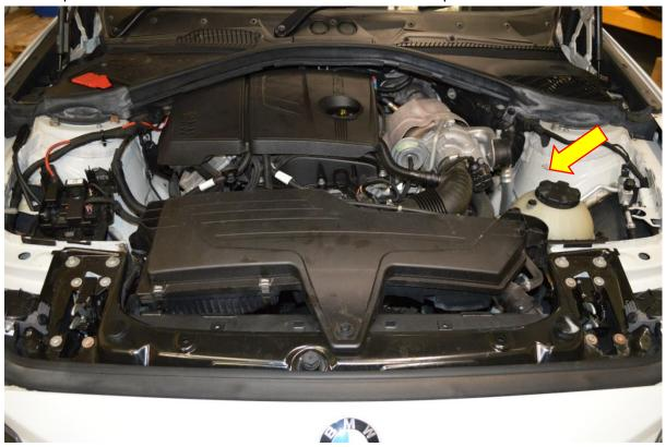
2. Using a T30 Torx drive remove three fasteners that hold the OEM valve in position and disconnect the wiring loom.
