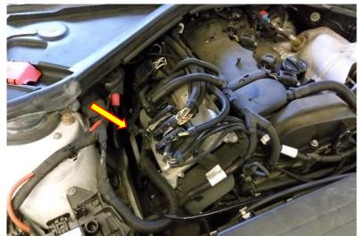
6. Using a 8mm socket and drive remove the fastener that holds the map sensor in position.
