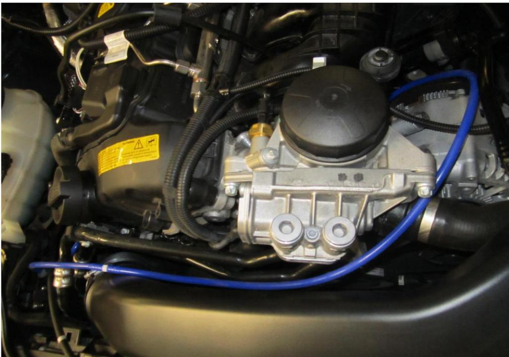
23. Connect this vacuum line to the solenoid on the port shown below
