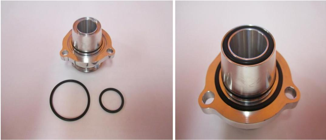
9. Fit your new dump valve into the original valves location. Once the fasteners have been tightened, replace the top on your forge valve making sure you put the spring in place.
