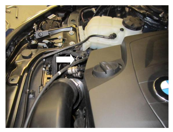
16. You now need to mount the solenoid provided with your new forge motorsport dump valve, we mounted it just behind the drivers light (RHD vehicle) where there is a spare hole available.
