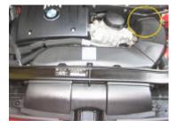
4.) Disconnect the small hose at the front of the air box. To remove this hose (circled below) simply squeeze the sides of the plastic ring connector and pull up. Then pull the hose away from the air box where it is held in place at the corner.
