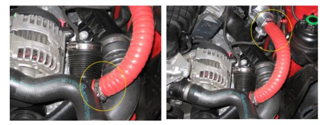
11B.) The procedure for the rear hose is the same. For this hose, it may be easiest to start by connecting it to the connection on the rearmost valve first (bottom left picture), and then connecting it to the rear port (bottom right picture).
