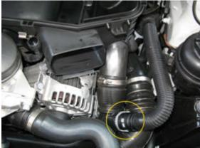
9.) Next, remove the vacuum lines from the factory diverter valves. These are the two small hoses that connect to the top center of each valve. To remove these, simply pull them away from the valve.
