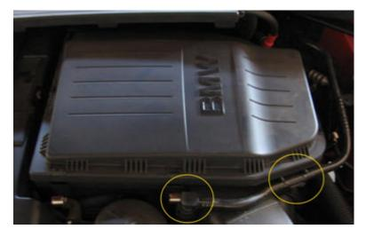
5.) Disconnect the two large intake hoses located at the front and rear of the air box (circled below). To remove simply use a flat head screw driver to loosen the clamp. Then, simply pull the hose free of the intake port on the air box.
