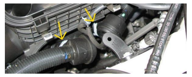
**10.**) With the factory diverter valves and hose out of the car, it is now time to install your Forge Motorsport diverter valves. You will want the small vacuum ports on the top of each valve to face the passenger side as shown below. See below for instructions on how to adjust these ports prior to installing the valves.
