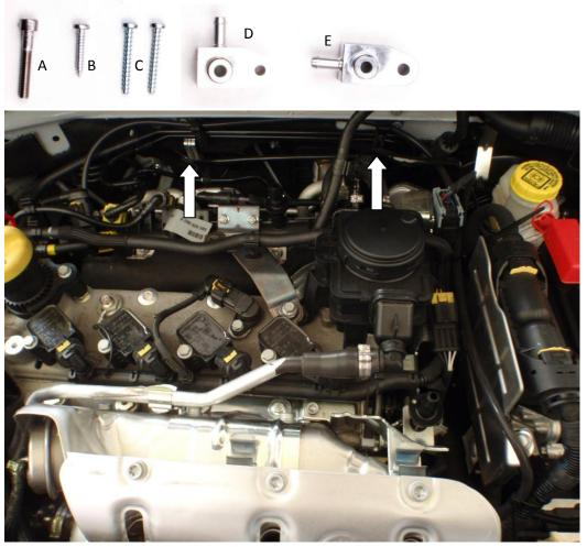
4. Connect the supplied length of silicon vacuum hose to the take off just fitted, and route it around the engine bay, using the clips already on the bulkhead to hold it in place, and route it between the ECU and the engine block to the front of the car by the stock valve. Use the supplied cable ties to secure it in the engine b
