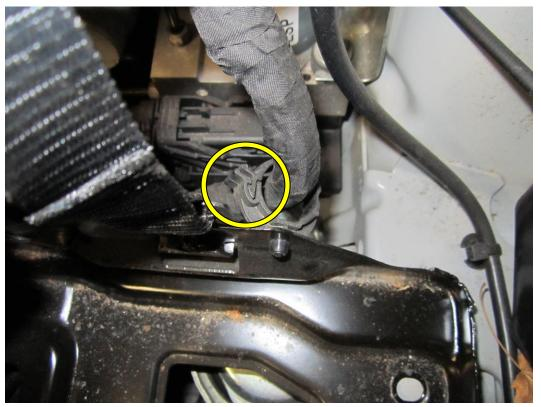
11. Now the battery tray has been completely removed locate the sensor that mounts on the boost pipe beneath. Using a T25 torx driver or 5mm Allen key, remove the sensor.
