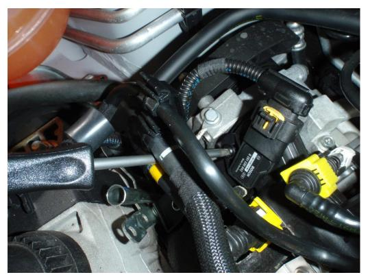
3. Place the Forge take off block **D** under the MAP sensor and push it securely in place, ensuring the o-ring is fitted to the take off. Screw the take off and MAP sensor as one unit back to the inlet manifold using supplied screw **C**. Place the supplied alloy spacer behind the plastic bracket and refit using supplied screw **B**.
