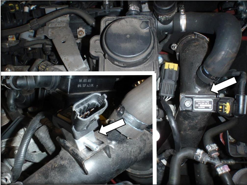
6. Undo the bolt from the MAP sensor on the inlet manifold and fit the spacer block with the vacuum pipe pointing to 12 o'clock. Reattach using the long screw with a Philips head supplied.
