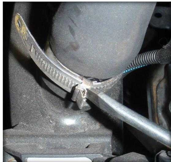
3. Remove the clip from the bottom part of the stock valve, undo the three bolts on the breather assembly and rotate to gain excess to the stock valve.
