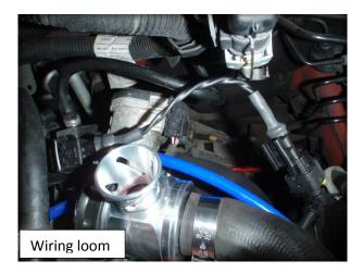
10. Attach the silicon hose blank to the filter pipe
