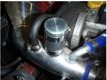
11. Remove the clips and hose from the engine cover and fit back to engine. Installation is complete.
