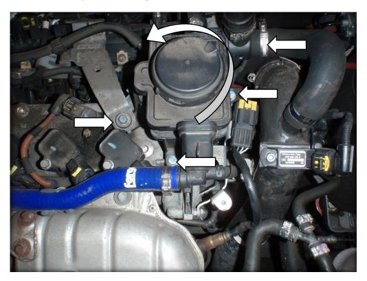
4. Undo the two bolts on the valve now having gained excess, unplug wiring loom and remove the stock valve and short hose still attached.
