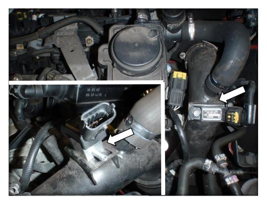
6. Undo the bolt from the MAP sensor on the inlet manifold and fit the spacer block with the vacuum pipe pointing to 12 o'clock. Reattach using the long screw supplied with a Philips head.
