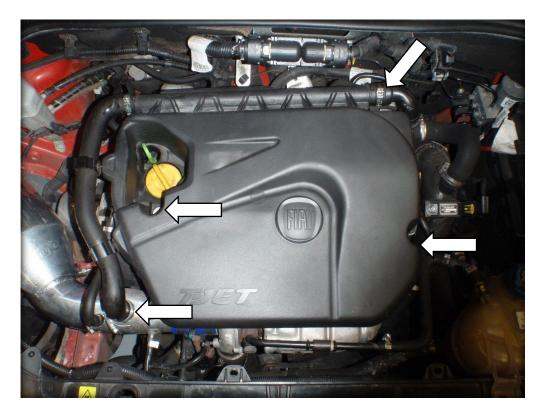
2. The clips on the hoses will need to be removed with a clip removing tool or breaking with a screw driver please see photos below.
