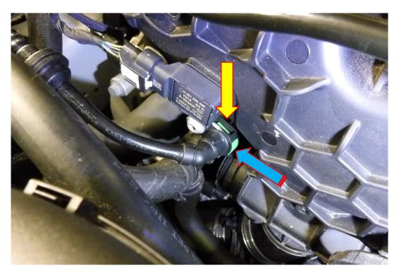
10. Take the supplied vacuum T piece adaptor and insert the smaller end into the vacuum pipe removed in the previous step. Now re fit the vacuum hose and adaptor back into place, once pushed as far as it will go, lock into position with the supplied retaining clip.
