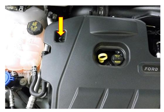
2. Remove X2 8mm fasteners attaching the intake pipe to the engine using an 8mm spanner or socket and rachet. Remove both breather hoses, the breather closest to the front of the vehicle simply unclips and the hose at the rear will need long nose pliers or a hose clamp removal tool to release it.
