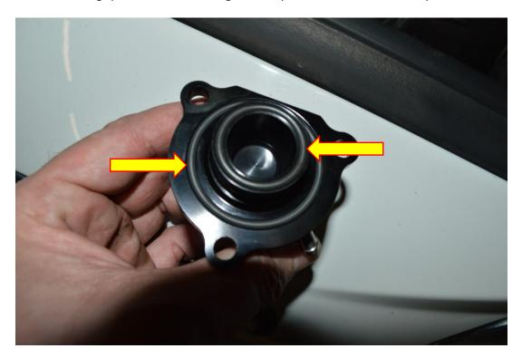
6. Fit the Forge Motorsport Valve with the X3 M6 Allen cap head bolts from the kit using a 5mm Allen key.
