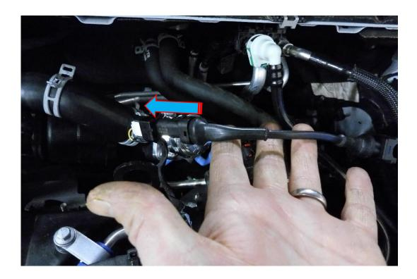
9. Remove the vacuum pipe located at the front of the inlet manifold. Push the green button inward and pull the pipe away at the same time, this will allow the vacuum pipe to come away.
