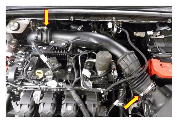
4. With the intake pipe now removed from the engine bay, you will now have better access to the OE valve. Unplug the wiring loom at the top of the valve, then remove the X3 M6 fasteners using a 4mm socket and rachet. The valve can now be removed from the boost pipe.
