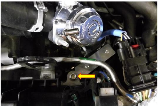
8. Fit the Forge wiring loom to the OE valve loom, make sure it is pushed all the way in until you hear it click. Route the other end of the Forge wiring loom to the solenoid, like before push the plug in until you hear it click into position.
