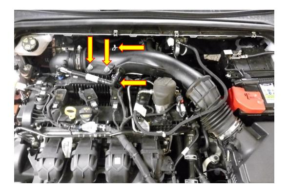
3. Loosen both hose clamps at each end of the intake pipe using a 7mm socket and rachet or flat blade screwdriver. You will now be able to pull the intake pipe out of the engine bay.
