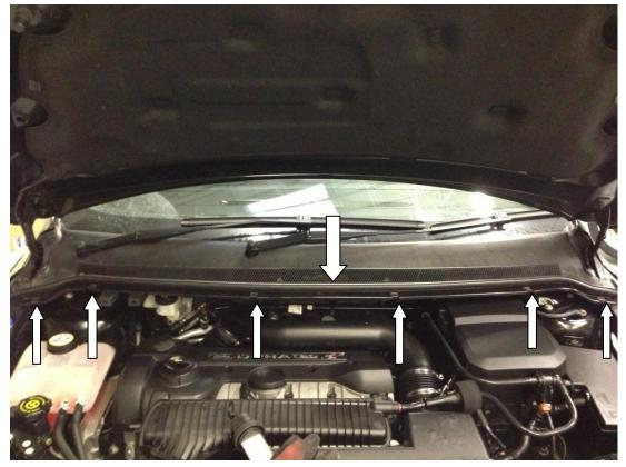
5. If you lift the scuttle panel you will see the other end of the noise generator pipe. This has a fixing on both sides holding it to the bulk head. To access these you will need to go under the bulk head into the engine bay and remove these using a Phillips screwdriver. This will now allow you to remove the noise generator. To do this simply lift the scuttle panel upwards and feed it out through the hole.
