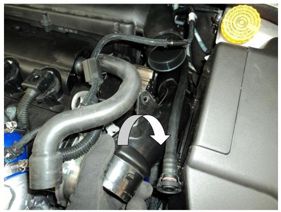
8. Undo the four T20 Torx holding the top of the air box to the bottom section. Then remove the top part of the air box.
