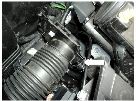
6. Rotate the other end of the pipe anti-clockwise to release the clip and remove this section of the cold air feed. Remove the 10mm bolt arrowed below (already removed in this pic)
