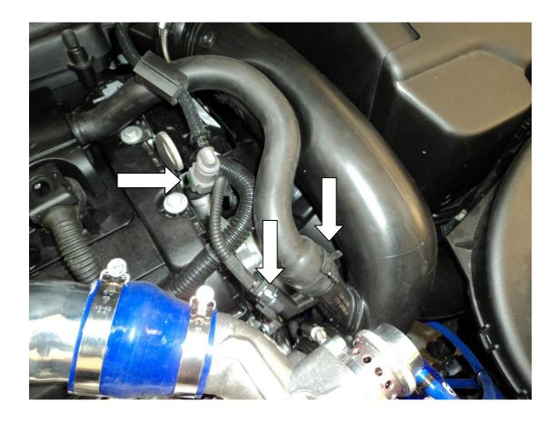
3. Release the secondry breather hose by squeezing the retianing tabs top and bottom and pulling the hose off towards the firewall – this can be tight as its held in place with two orings. Loosen the hose clip securing the pipe to the turbo with a 7mm hose clamp driver. Remove the turbo to airfilter intake pipe from the car.
