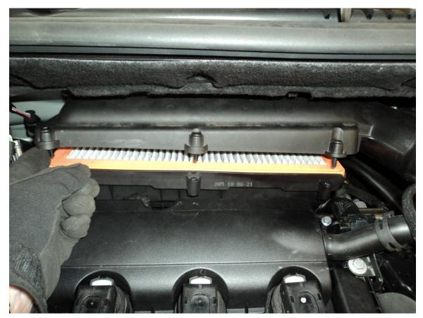
9. Remove the single T25 screw holding the airbox down on the far left behind the oil breather pipe.
