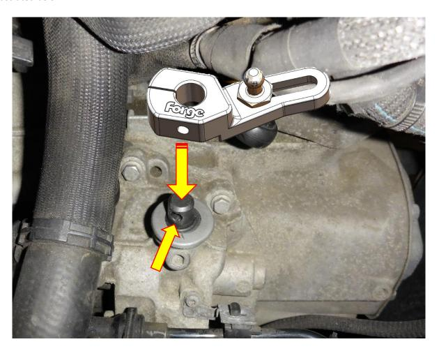
8. Using a 10mm socket and suitable driver and a 10mm spanner attach the supplied M6 bolt, washers and nyloc nut through the hole in the shifter and shaft to secure the shifter as detailed below.
