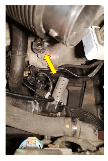
5. Pinch the white tabs on the selector cable and pull vertically to disconnect it from the mechanism.
