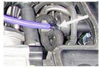
Insert "T" into vacuum line that leads to the fuel regulator
