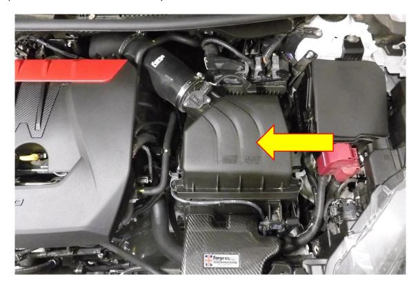
2. Un plug the loom from the MAF sensor and using a 10mm or 7mm socket and rachet loosen the hose clamp securing the inlet hose.
