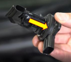
10. Position the MAF sensor into the hole in the airbox as shown in the image below. The arrow will point
