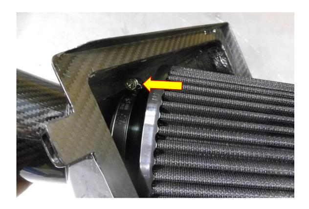
13. In the FMINDK43 kit are 2X silicone coupler hoses, one of which is a reducer for use with the OE intake pipe and the other an 89mm straight coupler for use with our FMTIA8 product. Slide the appropriate coupler into position with the two supplied hoses clamps loosely.
