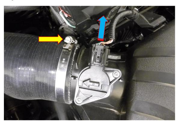
3. The MAF loom is attached to the top of the OE air box, using a trim tool or flat blade screwdriver prise the loom away from the air box.
