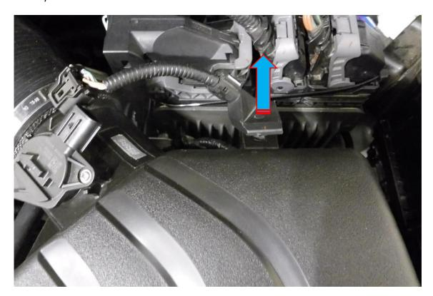
4. Release the retaining clips at the front of the air box.
