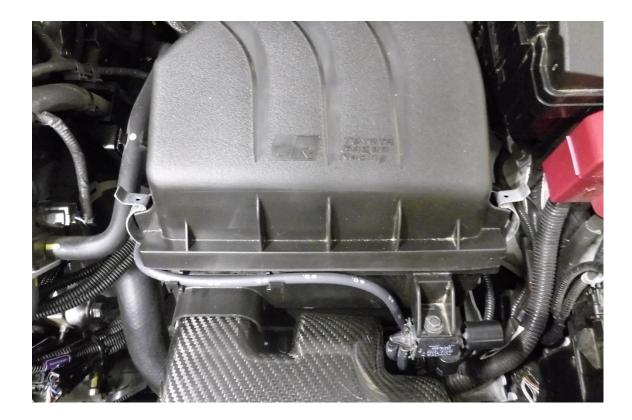
5. Remove the air box lid from the engine bay.
