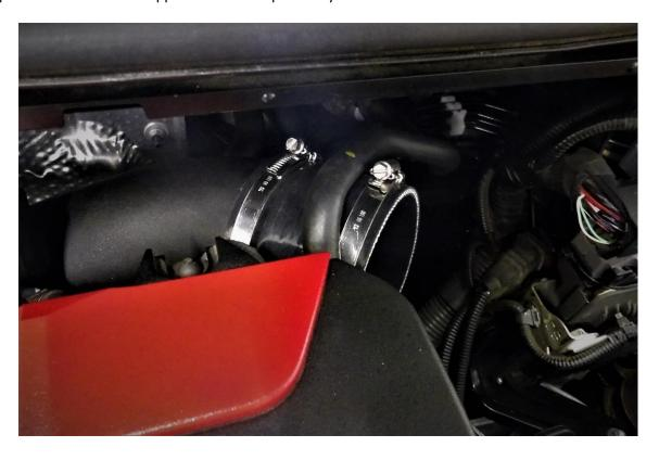
14. Insert the inlet pipe section of the FMINDK43 into the silicone joiner and slide the mounting lugs are located into the bottom part of the OE air box. Tighten the hoses clamps to 2-2.4nm secure the silicone coupler, now follow steps 1-4 in reverse order.
