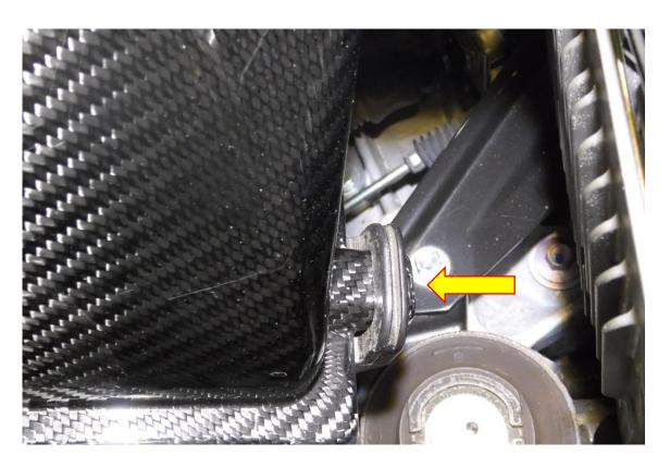
15. Finally use the supplied cable tie to secure the MAF loom to the ECU loom as shown in the picture below. This is the installation of FMINDK43 complete, make sure to give the vehicle a final spanner check and enjoy your new Forge Motorsport product.
