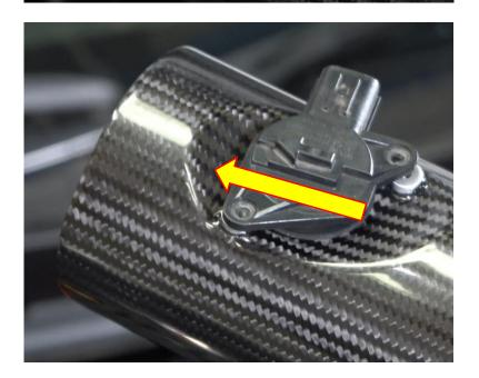
**11**. Using a 3mm Allen key secure the MAF sensor to the Forge Motorsport airbox lid using the **SUPPLIED M5** fasteners please do not over tighten, these should be only torqued to 0.8NM and no more than 1NM.
