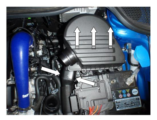
5. Undo the T25 screws holding the cold air feed and remove then undo the T30 torx screws on the turbo hosing holding the resonator pipe and remove.
