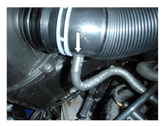
4. Remove the air filter by unclipping the cold air feed and pulling upwards releasing it from the rubber grommets.
