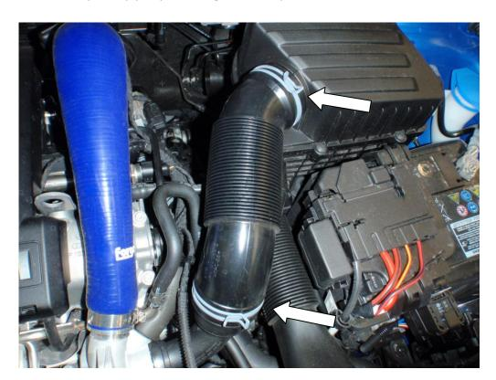
3. Before the pipe can be taken off remove the vacuum hose. You may need to use a screw driver to pry it off.
