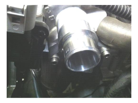
7. Insert the aluminium tube into the silicon hose making sure not to block off the vacuum port and secure with JCS clip. Then Push the filter over the aluminium tube and secure with the JCS clip.
