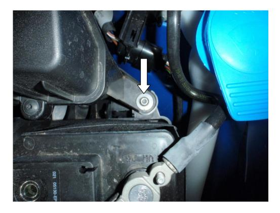
2. Remove the plastic pipe by removing the two clips.
