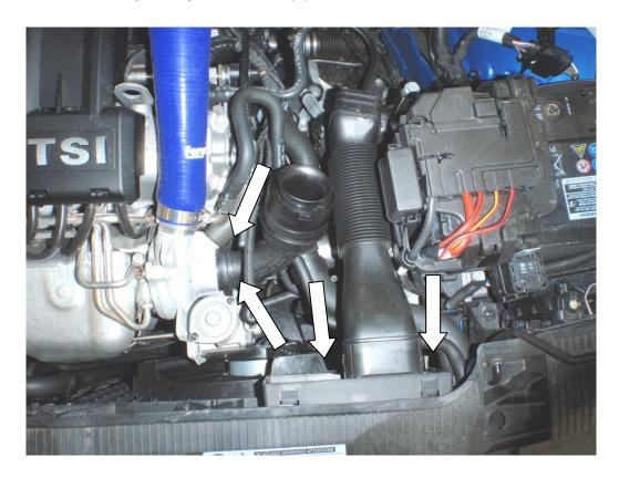
6. Connect the supplied turbo inlet connector using the supplied 5mm Allen head bolts.
