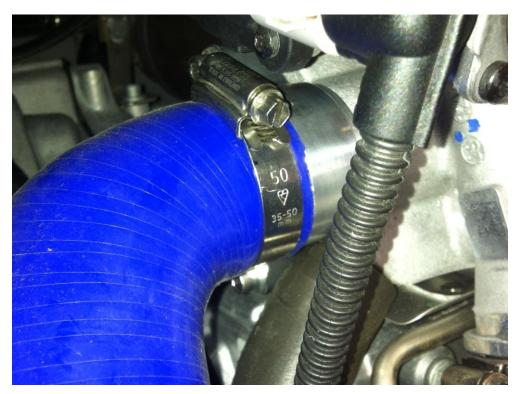
10. Connect the vacuum pipe to the silicon hose using the small aluminium tube and JCS clips.
