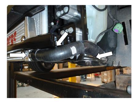
25. Push the long silicon hose onto the intercooler with a 55mm jubilee clip and do up in such a way that the bulky part of the clip is not on the bottom of the pipe as the intercooler sits slightly lower than stock. The silicon should be tight against the crash bar and going over the bracket of the old intercooler.
