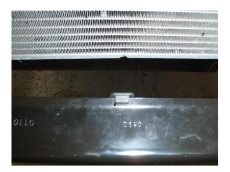
18.Looking down on the crash bar you will see three clips holding the washer bottle hose in position remove these with your screw driver.
