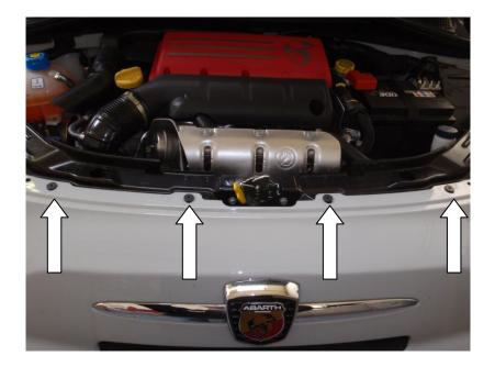
7. Undo the last four T30 screws taking care as there will be nothing holding the bumper on, once the screws are removed gently pull the bumper away from the car and place to one side.
