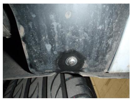
3. Looking under the car up at the arch liner there is a pozidriv/Phillips screw, undo this on both sides of the vehicle.
