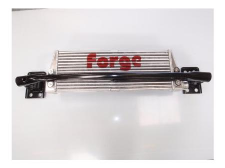
21. Fit the intercooler loosely to the new crash bar using the 4 M6 bolts and 4 penny washers.
