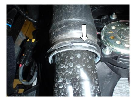
12.Looking up you will see where the pipe joins in the middle going up to the rubber hose joining it to the inlet manifold pull this clip off, now the pipe is free to be removed completely.
