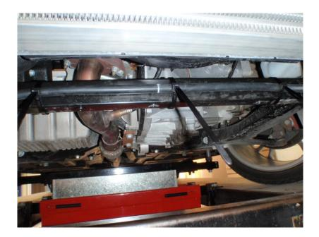
20. Using the zip ties supplied in the kit reattach the washer bottle hose to the chassis as above. Your Abarth is now ready to start fitting the upgraded intercooler!
