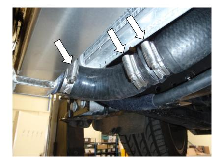
24. Push the coupler into the stock rubber hose and tighten a 50mm jubilee clip around the rubber hose, put the two remaining 50mm jubilee clips on the 90 degree silicon hose before installing, and then push the short leg of the 90 degree silicon joiner onto the intercooler and the long leg into the coupler. Now tighten the 50mm jubilee clips on the silicon hose.
