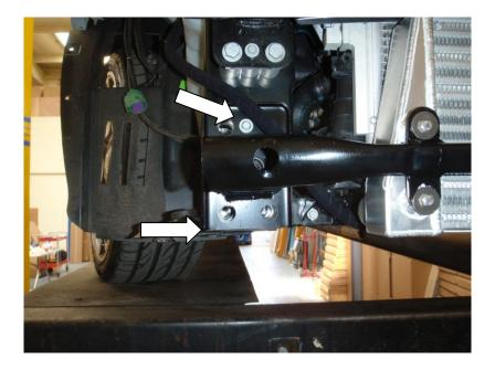
22. Using the two 10mm bolts reattach the crash bar lining the spacers up and keep a 5mm gap between the bottom of the crash bar and the top of the chassis. When the crash bar is in the correct position replace the eight 17mm bolts.
