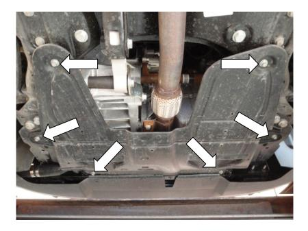
4. Undo the six 10mm bolts on the under tray using a 10mm socket and ratchet and remove.
