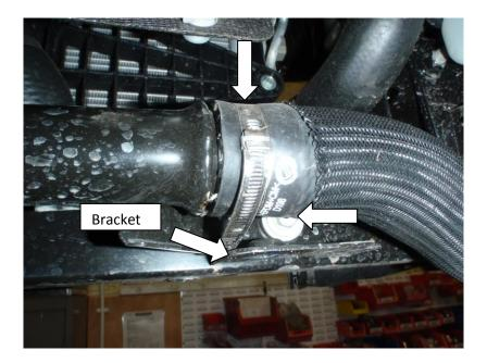
11. Looking at the driver's side of the pipe again the use 'once only' clip must be broken, remove the 10mm bolt and keep bracket to one side to be replaced after pipe is removed
