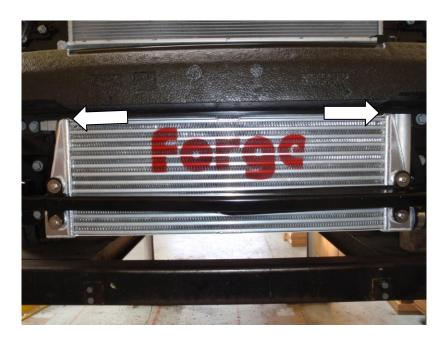
23.Push the intercooler upwards until it is flush with the upper crash bar and tighten up the four 10mm bolts.
