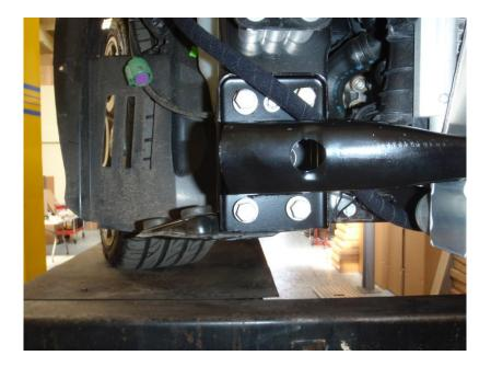
19. Undo the four 17mm bolts and the one 10mm bolt retaining the crash bar. Repeat on the other side and remove the crash bar from the car.
