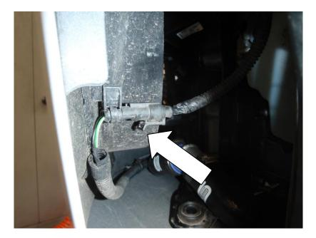
2. Additionally on the left hand side you will need to pull back the arch liner. You should see another connecter (see above). Pull the clip down and pull away to disconnect.
