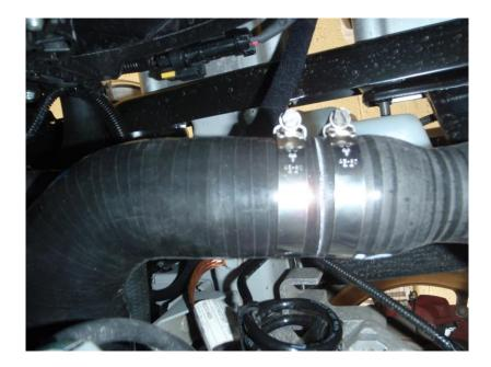
26. Push the 45mm diameter joiner in the other end of the long silicon hose you have just fitted, and tighten the jubilee clip. With the remaining silicon hose loosely fit the 70mm and 55mm jubilees clips, push the large end on the existing plastic pipe (see photo below) and connect the other end to the joiner and do up the jubilee clips. Follow points 1-7 in reverse order to refit the bumper, installation is complete!
