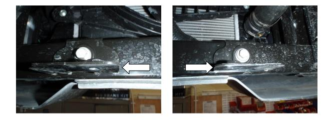
14. The brackets that were taken off with the metal pipe in steps 10 + 11 need to be replaced with the original bolts.
