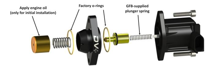
Note that the bolt holes are NOT SYMMETRICAL. When you assemble the DV+body onto the solenoid body, check the alignment of the holes - if they do not line up properly, rotate the DV+body 180 degrees and check that they line up correctly before installing on the car.
