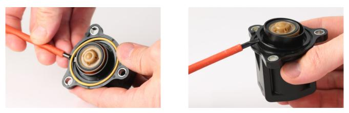
Assemble the GFB parts onto the factory solenoid body as shown in the exploded view below, making sure to use the GFB-supplied plunger spring, and the yellow o-ring removed from the factory valve. Apply some engine oil to the piston during this process. Note that regular re-lubrication is NOT required.
