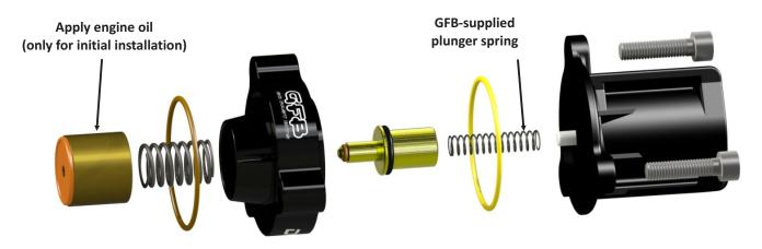
During assembly, check that the piston slides freely in the body without sticking or binding. It is a very close fit and can sometimes be difficult to get started into the bore, but once in it should move without needing to be forced.
