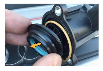
Check the fit of the piston in the DV+ body. It is a very tight tolerance and can sometimes be tricky to get started into the bore. Once inserted, it should slide freely without sticking.
