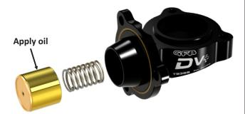
Hold the piston to prevent it from falling out, then install the DV+ body onto the turbo.
