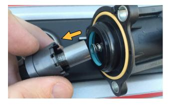
Remove the plastic piston shroud from the solenoid. This should be able to be removed by hand, but if it does need to be levered out take care not to damage any of the plastic pieces. Store the piston, shroud and spring safely as these are not used, and keep the yellow o-ring and bolts for the DV+ installation.
