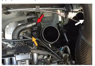
Using a Torx T30 driver, loosen the single screw (yellow arrow) that retains the hard plastic turbo intake elbow. This screw usually has an o-ring under it to prevent it from falling out as it is loosened, but take care not to drop it anyway.
