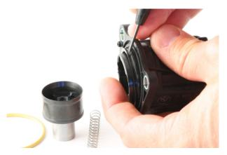
Assemble the GFB parts onto the factory solenoid body as shown in the exploded view below, making sure to use the GFB-supplied plunger spring, and the yellow o-ring removed from the factory valve. Apply some engine oil to the piston during this process. Note that regular re-lubrication is NOT required.
