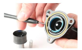
CAREFULLY pry the piston sleeve out of the diverter body, using the inside lip near the blue seal or the lip where the o-ring was. Lever it gently and work your way around so it pops out evenly.
