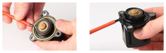
Assemble the GFB parts onto the factory solenoid body as shown in the exploded view below, making sure to use the GFB-supplied plunger spring, and the yellow o-ring removed from the factory valve. Apply some engine oil to the piston during this process, and check that the piston moves freely.
