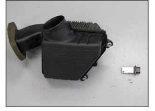
11. Remove the two screws securing the mass air sensor into the factory air box and then remove the sensor from the air box.
