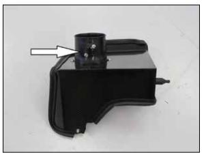
12. Install the mass air sensor into the K&N<sup>®</sup> mass air sensor housing and secure with the provided hardware.
