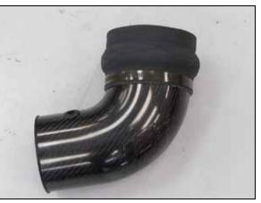
16. Install the provided hump hose (08695) onto the K&N<sup>®</sup> intake tube and secure with the provided hose clamp.
