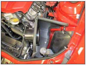
13. Install the heat shield into the engine compartment so the mounting stud inserts into the air box mount grommet and the mounting bracket installs onto the mounting stud.
