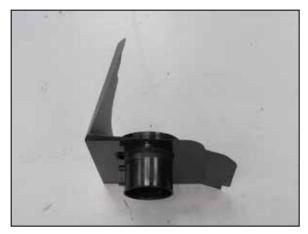
7. Install the K&N $^{\otimes}$  mass air sensor adapter into the heat shield and secure with the provided hardware.
