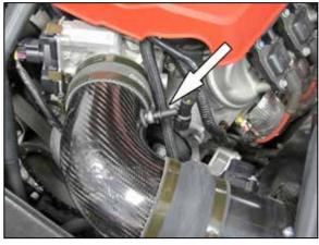
19. Install the provided crank case vent fitting into grommet in the  $K\&N^{\otimes}$  intake tube as shown.
