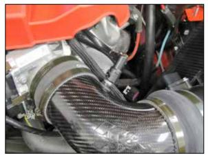
20. Rotate the crank case vent fitting clockwise and then connect to the fitting installed into the K&N<sup>®</sup> intake tube in the previous step.
