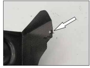
Install the heat shield mounting bracket (070066) onto the heat shield as shown.
