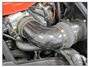
18. Install the K&N<sup>®</sup> intake tube assembly into the silicone hose at the throttle body and then install the hump hose onto the mass air sensor housing. Secure the tube with the provided hose clamps.
