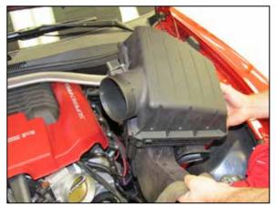
6. Remove the air box from the vehicle. NOTE: K&N Engineering, Inc., recommends that customers do not discard factory air intake.
