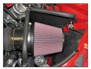
22. Install the K&N<sup>®</sup> air filter and secure with the provided hose clamp.
