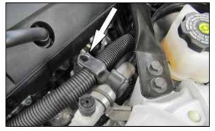
8. Disconnect the mount securing the sound tube to the A/C line.
