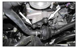
6. Remove the two bolts securing the sound drum to the front of the engine.
