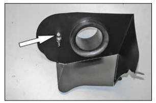
15. Install the provided mounting bracket assembly onto the heat shield using the provided hardware.
