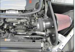
23. Install the K&N<sup>®</sup> air filter onto the filter adapter and secure with the provided hose clamp. NOTE: Drycharger<sup>®</sup> air filter wrap; part # RF-1042DK is available to purchase separately. To learn more about Drycharger<sup>®</sup> filter wraps or look up color availability please visit http://www.knfilters.com<sup>®</sup>.
