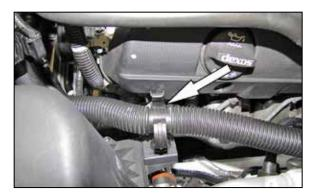
7. Open the clamp securing the sound tube to the air filter housing.
