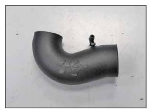
24. Install the provided 90° fitting into the K&N<sup>®</sup> intake tube as shown.
