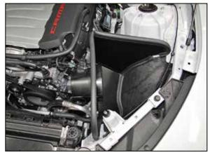
20. Install the K&N<sup>®</sup> heat shield assembly onto the air filter housing mounting grommets.
