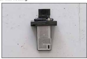
15. Install the mass air sensor into the K&N® mass air sensor adapter and secure with the provided hardware.
