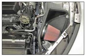
10. Install the heat shield/filter assembly into the vehicle so the mounting studs insert into the mounting grommets.
