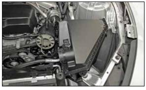
4. Lift the air filter housing to dislodge it from mount grommets and then remove the housing from the vehicle.
