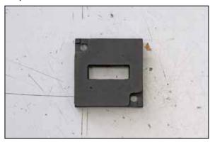
13. Install the provided gasket onto the bottom of the mass air sensor adapter.
