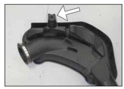
19. Remove the intake plenum mounting grommet from the intake plenum.
