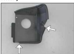
11. Install the provided shorter edge trim onto the bottom of the heat shield as shown.
