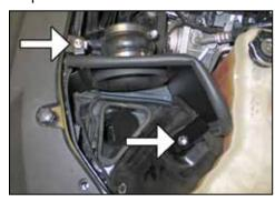
14. Install the heat shield assembly onto the inner fender; secure the mounting bracket to the factory air box mounting location and secure with the provided hardware. Place the insert nut into the hole in the inner fender and tighten the bolt to secure.
