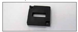
10. Install the provided gasket onto the K&N<sup>®</sup> mass air sensor adapter.
