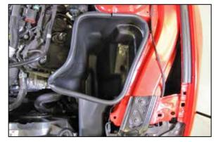
8. Install the provided edge trim onto the K&N<sup>®</sup> air filter housing. Install the K&N<sup>®</sup> air filter housing into the vehicle and secure with the provided hardware. **NOTE: Some trimming of the edge trim will be necessary.**
