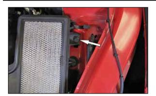
7. Remove the bolt that secures the air filter housing to the inner fender and then remove the lower air filter housing from the vehicle. **NOTE: K&N Engineering, Inc., recommends that customers do not discard factory air intake.**
