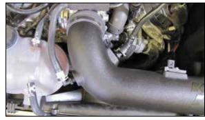
16. Connect the EVAP and crank case vent lines to the fittings installed into the K&N<sup>®</sup> intake tube.
