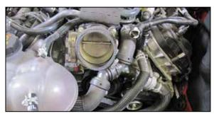
13. Install the provided coupling hose (08699) onto the throttle body and secure with the provided hose clamp.
