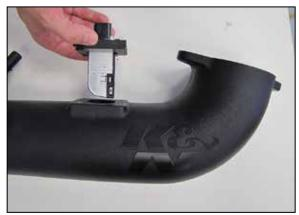
12. Install the mass air sensor assembly into the  $K\&N^{\ensuremath{\circledast}}$  intake tube as shown and secure with the provided hardware.
