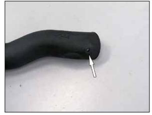
17. Install the provided grommet into the  $K\&N^{\otimes}$  intake tube as shown.
