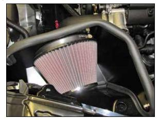
14. Install the K&N<sup>®</sup> air filter onto the filter adapter and secure with the provided hose clamp. NOTE: Drycharger<sup>®</sup> air filter wrap; part # 22-8049DK is available to purchase separately. To learn more about Drycharger<sup>®</sup> filter wraps or look up color availability please visit http://www.knfilters.com<sup>®</sup>.
