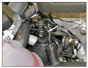
21. Connect the crank case vent hose to the fitting installed into the  $K\&N^{\otimes}$  intake tube.
