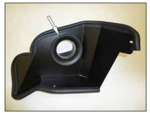
10. Install the filter adapter into the heat shield as
