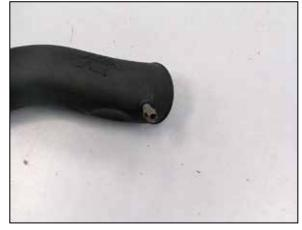
18. Remove the O-Ring from the factory temperature sensor and then install the sensor into the grommet installed into the K&N<sup>®</sup> intake tube.
