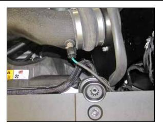
23. Connect the provided extension harness to the factory inlet air temperature sensor harness and then connect the other end to the inlet air temperature sensor as shown.
