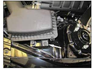
8. Remove the bolt securing the air filter housing to the inner fender and remove the air filter housing from the vehicle
