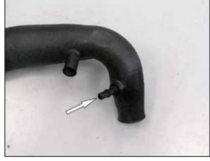
19. Install the provided quick disconnect fitting into the K&N^ $\!\!^{\textcircled{\sc on}}$  intake tube as shown.
