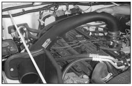
19. Install the K&N® intake tube.
