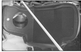
16. Install the heat shield assembly.
