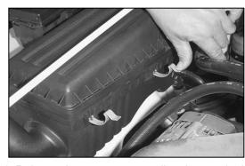
4. Release the 5 over center clips that retain the air box top to the air box base.
