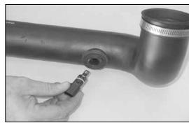
5. On vehicles equipped a with temperature sensor, lift the temperature sensor-locking tab while twisting the sensor counter clockwise to remove the sensor from the intake tube. **NOTE:** The temperature sensor is fragile,
