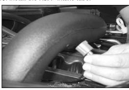
19a. Position the temperature sensor electrical connector next to the K&N $^{\odot}$  intake tube for the best fit, then mark the location to be drilled.
