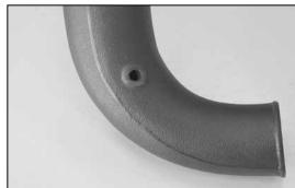
19b. Remove the K&N $^{\circ}$  intake tube from the vehicle and drill a 3/4" hole at the position marked in step #19a. Install the provided grommet into the hole that was drilled out.
