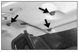
7. Loosen and remove the 3 nuts that retain the air box base to the inner fender apron.
