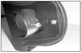
15. Attach the saddle bracket assembly to the heat shield using the provided hardware.
