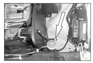
10. Using the provided hardware, secure the "L" bracket to the inner fender as shown.
