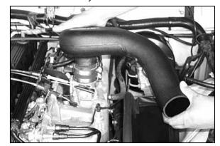
13. Install the K&N® intake tube onto the throttle body and tighten the hose clamp.
