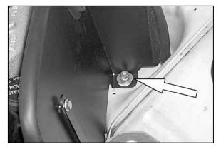
11. Using the provided washers and the hex nut removed in step 5, secure the heat shield assembly to the existing stud as shown.
