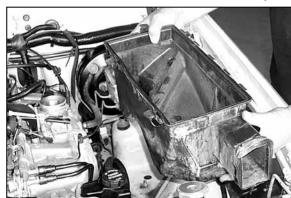
6. Remove the lower air cleaner assembly as shown
