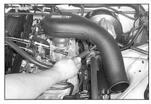
14. Install the provided silicone hose onto the crankcase vent, then install the other end onto the K&N® intake tube
