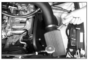
16. Install the K&N® Filtercharger onto the K&N® intake tube as shown.
