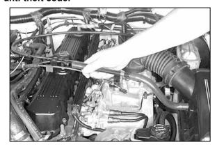
2. Remove the crankcase vent line from the valve cover.
