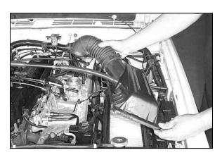
4. Loosen the hose clamp at the throttle body and unclamp the airbox lid then remove the upper intake assembly as shown.
