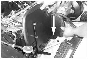
9. Install the heat shield assembly into the vehicle lining up the factory stud with the tab on the heat shield.
