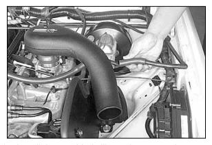
15. Install the provided silicone hose onto the EVAP canister vent line then secure the other end onto the K&N® intake tube.
