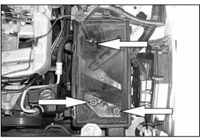
5. Loosen and remove the two bolts and one hex nut that secure the lower air cleaner assembly.
