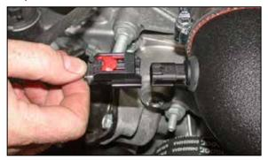
23. Reconnect the air temperature sensor electrical connection as shown.
