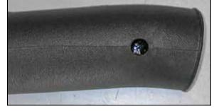
16b. Drill out the hole in the intake tube to 0.75".
