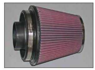
20. Install the filter adapter into the air filter and secure with the provided hose clamp.
