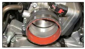
14. Install the silicone hose (08630) onto the throttle body and secure with the provided hose clamp as shown.
