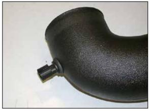
17. Install the factory air temperature sensor into the grommet installed in step #16.
