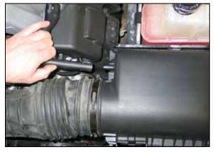
5a. On SRT-8; 6.1L vehicles, disconnect the crank case vent hose from the air box as shown.
