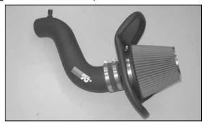
18. Install the air filter assembly onto the K&N® intake tube as shown.
