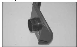
10. Install the air filter adapter onto the heat shield with the provided hardware as shown.
