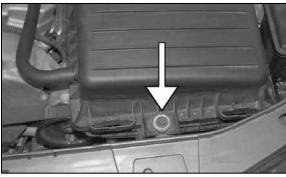
5. Loosen and remove the airbox mounting bolt as
