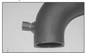
15. Install the air temperature sensor into the grommet installed in step #14.
