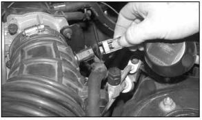
2. Unlock the red locking tab on the air temperature sensor electrical connection, then depress the locking lever and pull apart the temperature sensor electrical connection
