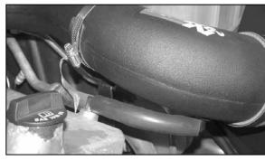
21. Install the provided silicone vent hose onto the valve cover vent and onto the elbow into the K&N® intake tube as shown.
