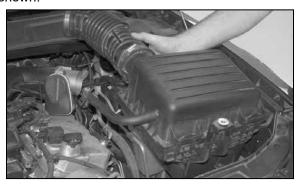
6. Lift the complete intake and air filter assembly to remove it from the vehicle.
