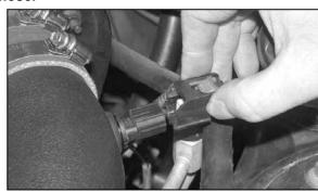
22. Reconnect the air temperature electrical connection as shown.
