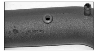
26. Install the supplied rubber grommet into the  $K\&N^{\ensuremath{\$}}$  intake tube as shown.
