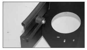
12. Install the bracket/rubber mounted stud assembly onto the heat shield as shown using the provided hardware.
