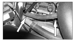
31.Install the supplied silicone hose onto the crankcase vent "T" and connect the other end onto the K&N<sup>®</sup> intake tube as shown. NOTE: Some vehicles may not have the described "T" fitting, the crank case vent fitting will be attached directly to the valve cover.
