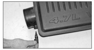
25. Rotate the air temperature sensor counter clockwise and remove the sensor from the stock intake plenum as shown.
