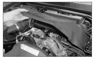
2. On 2008 and later model vehicles, pull up on the engine cover to dislodge it from the mounting grommets and then remove the engine cover from the vehicle. 2a. Loosen the hose clamp, which secures the stock intake tube to the intake plenum, and disconnect the crankcase vent hose from the airbox lid.
