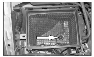
8. Remove the airbox mounting bolt shown.
