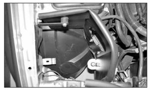
19. Install the heat shield assembly into the vehicle and secure it to the mounting locations with the provided hardware.
