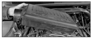
20c. Remove the intake plenum from the vehicle as shown.
