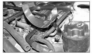
24. Install the tube mounting bracket assembly onto the A/C compressor and secure with the factory-mounting bolt removed in step #23.
