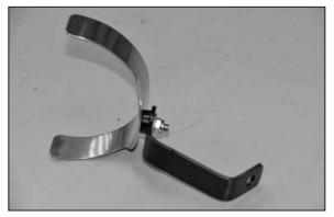
22. Install the saddle clamp onto the tube mounting bracket and secure with the provided hardware as shown.
