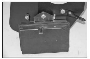
15. Using the provided spacer, install the vacuum reservoir onto the heat shield as shown. NOTE: Due to vehicle manufacturing tolerances, 2 spacers may be required. NOTE: Some vehicles may not be equipped with a vacuum reservoir.
