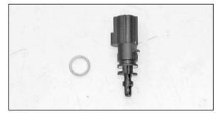
27. Remove the rubber sealing "O" ring from the air temperature sensor as shown.
