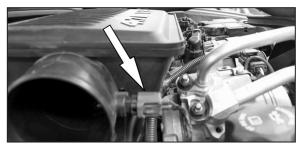
20a. Disconnect the air temperature electrical connection.
