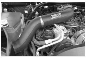
29. Install the K&N<sup>®</sup> intake tube into the silicone hose at the throttle body and onto the saddle clamp, then secure with the provided hose clamps as shown.
