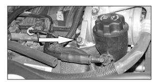
23. Remove the Lower rear A/C mounting bolt shown.
