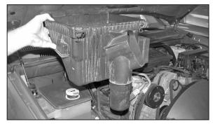
9. Lift the lower airbox and remove it from the vehicle as shown.
