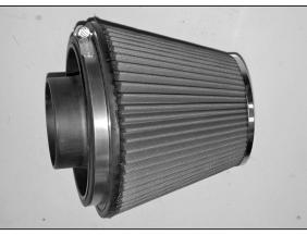
32. Install the filter adapter into the air filter as shown, secure with the provided hose clamp.
