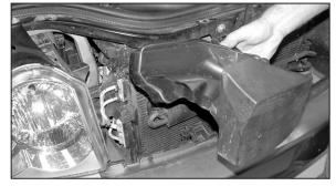
7. Pull the fresh air duct forward to disconnect it from the airbox and then remove it from the vehicle.
