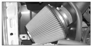
34. Install the air filter assembly onto the K&N<sup>®</sup> intake tube as shown and secure with the provided hose clamp.
