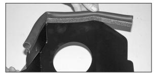
10. Install the provided edge trim onto the heat shield as shown.
