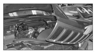
6. Remove the six grill retaining clips from the grill, then tilt the grill forward and lift to remove from the vehicle.
