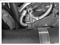
32. Reconnect the air temperature sensor electrical connection as shown.
