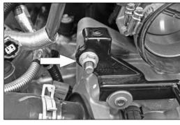
23. Remove the nut, which secures the intake plenum-mount shown.
