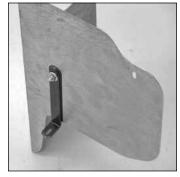
16. Install the large "L" bracket (26626) onto the heat shield as shown with the provided hardware.
