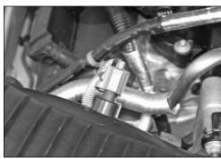
6. Disconnect the air temperature sensor electrical connection and then remove the intake plenum from the vehicle.
