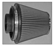
33. Install the filter adapter into the air filter as shown, secure with the provided hose clamp.
