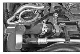
25. Install the tube mounting bracket assembly onto the plenum mount and secure with the factory nut removed in step #23.
