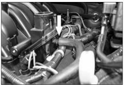
8. Remove the crank case vent hose from the engine as shown.
