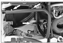
21. Install the heat shield assembly into the vehicle and secure to the lower and upper air box mounts and washer bottle stud with the provided hardware.
