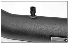
29. Install the air temperature sensor into the intake tube as shown.
