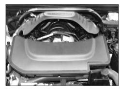
3. Remove the oil filler cap and then lift up the front of engine cover to gain access to the throttle body hose clamp intake plenum mounting bolt.
