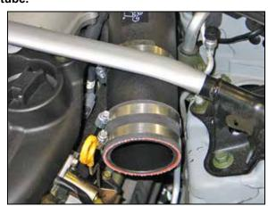
19. Install the silicone hose (08690) onto the end of the K&N® intake tube with the provided hose
