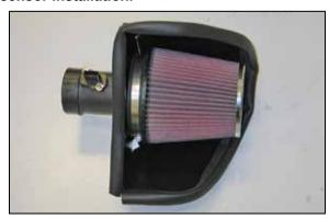
20. Install the Air Filter onto the radius filter adapter
