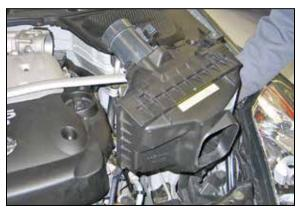
6. Lift up on the air box to dislodge it from the mounting grommet and then remove the air box from the vehicle as shown.
