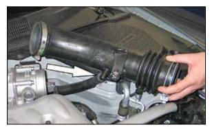
4. Loosen the two hose clamps, which secure the stock intake tube to the throttle body and air box. Then lift the intake tube up to access the crank case vent hose and disconnect the vent hose from the intake tube. Next remove the intake tube from the vehicle.
