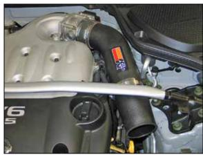
18. Install the K&N® intake tube onto the throttle body and saddle clamp and then secure with the provided hose clamps as shown.
