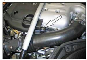
3. Remove the bolt, which secures the stock intake tube to intake manifold.
