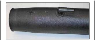
16. Install the provided 90 deg. fitting into the grommet that was installed onto the K&N® intake tube in step #15.
