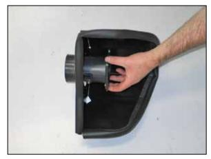
10. Pass the mass air sensor housing through the heat shield as shown.
