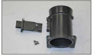
9. Remove the two screws, which secure the mass air sensor into the mass air housing, then remove the mass air sensor from the housing.
