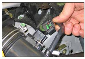
2. Depress the locking tab and disconnect the mass air sensor electrical connection. Next separate the mass air sensor wire harness from the clips, which attach to the air box.
