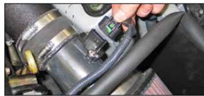
22. Reconnect the mass air sensor electrical connection and secure the wiring harness to the heat shield in the hole provided.
