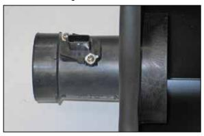
12. Reinstall the mass air sensor into the mass air sensor housing with the factory screws removed in step #9.
