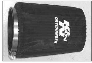
24. Install the provided  $K\&N^{\$}$  Drycharger $^{\$}$  onto the  $K\&N^{\$}$  air filter as shown.
