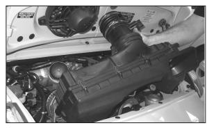
7. Pull up firmly, removing the factory air box and intake tube as shown.
