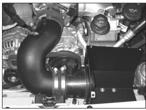
19. Install the K&N® intake tube onto the throttle body and mass air sensor housing. Secure with the provided hose clamps as shown.
