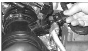
2. Depress the locking tab, then disconnect the mass air sensor electrical connection.
