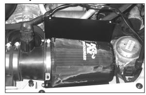
25. Install the K&N® air filter onto the K&N® intake tube and secure with the provided hose clamp as shown.
