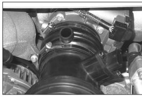
6. Loosen the hose clamp securing the factory intake tube to the throttle body as shown. Pull the factory intake tube from the throttle body.
