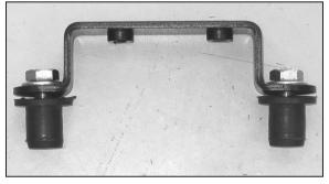
16. Assemble heat shield bracket (#26660) and threaded inserts with the provided hardware as shown.
