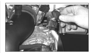
22. Pull the rubber wiring harness boot back from the mass air sensor electrical connector as shown. Rotate the connector 180 degrees and re-install the boot.
