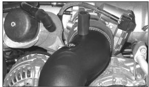
20. Install the provided silicone hose onto the  $K\&N^{\otimes}$  intake tube as shown.
