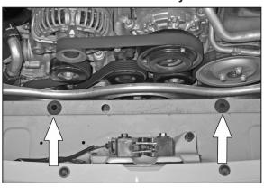
8. Remove the two air box mounting grommets as shown.
