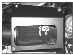
27. Install the heat shield top cover and mass air sensor harness clip (removed in step # 4) onto the heat shield with the provided hardware as shown.
