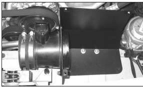
18. Install the heat shield assembly onto the heat shield bracket with the provided hardware as shown.
