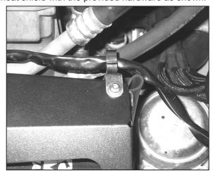
28. Re-attach the mass air sensor harness into the mass air sensor harness clip (mounted on heat shield) as shown.
