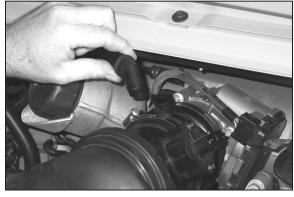
5. Remove the crank case vent line from the factory intake tube as shown.
