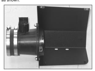
14. Install silicone hose (#08536) onto the mass air sensor housing and secure with the provided hardware as shown.
