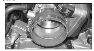
14. Install the silicone hose (08630) onto the throttle body and secure with the provided hose clamp as shown.
