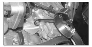
13. Using the provided spacer, install the tube mounting bracket assembly onto the engine as shown.
