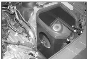
11. Install the heat shield assembly into the vehicle and secure to the bracket installed in step #8. Then secure the "L" bracket with the factory bolt removed in step #6 to the airbox mounting location.
