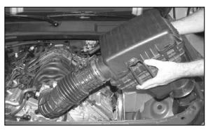
7. Lift the complete intake and air filter assembly to remove it from the vehicle.
