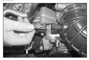
3. Unlock the red locking tab on the air temperature sensor electrical connection, then depress the locking lever and pull apart the temperature sensor electrical connection.
