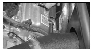
19. Install the provided crank case vent hose onto the vent port on the valve cover then install the vent hose onto the K&N® intake tube. NOTE: Due to manufacturer changes over time, It may be necessary to use the 5/8 to 1/2 " union fitting and 5/8" CCV hose connected to the ½" CCV hose.
