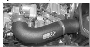
18. Install the K&N® intake tube into the throttle body and onto the saddle clamp as shown, then secure with the hose clamps provided.
