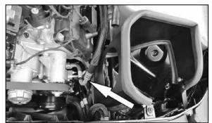
11a. Due to vehicle manufacturing tolerances, the A/C lines on some vehicles may need to repositioned slightly so that they do not contact the heat shield. To adjust, grab the A/C line on the aluminum section and carefully apply pressure in the desired direction until clearance is obtained.
