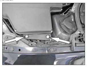
4. Remove the two bolts securing the factory air box to the inner fender.
