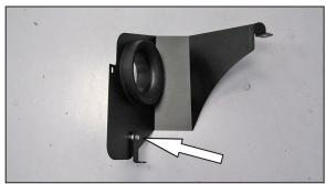
8. Install the heat shield mounting bracket (083170) onto the heat shield and secure with the provided hardware.
