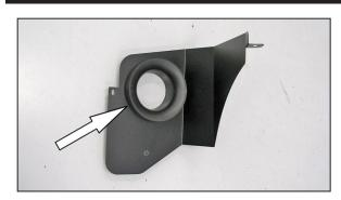
7. Install the filter adapter into the K&N® heat shield and secure with the provided hardware.
