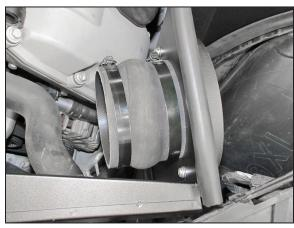
15. Install the provided coupling hose (08418) onto the filter adapter and secure with the provided hose clamp.
