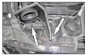
19. Secure the heat shield to the air filter housing studs with the provided hardware.
