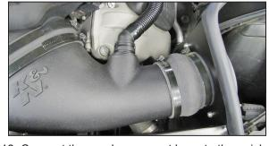
18. Connect the crank case vent hose to the quick disconnect fitting on the K&N® intake tube.
