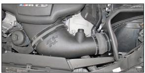
17. Install the K&N® intake tube into the hose at the filter adapter and then align with the throttle body. Slide the hose back onto the throttle body, align the tube for best fit and then secure the hose clamps.
