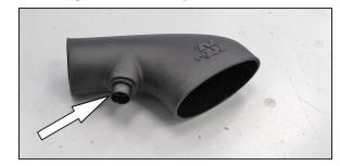
14. Install the provided grommet and quick disconnect fitting into the K&N® intake tube as shown.
