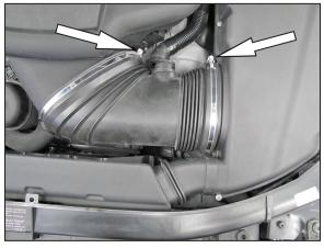
3. Loosen the Hose clamps securing the intake hose and then remove the intake hose from the vehicle.
