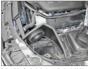
13. Install the fresh air duct onto the heat shield and secure with the provided hardware then install the heat shield assembly onto the air filter housing mounting studs but do not secure at this time. NOTE: The K&N® fresh air duct will insert into the factory fresh air scoop.
