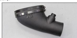
16. Install the provided coupling hose (08619) onto the K&N® intake tube and slide it as far as possible on.
