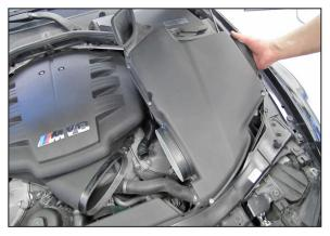
5. Lift up the factory air filter housing and fresh air intake duct and remove them from the vehicle.
