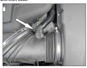
2. Release the locking ring securing the crank case vent to the intake tube and then disconnect the crank case vent hose from the intake tube
