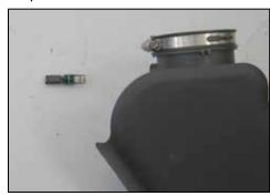
16. Rotate the inlet air temperature sensor counter clockwise and then remove from the factory intake tube.
