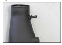
17. Install the provided grommet and inlet air temperature sensor into the K&N® intake tube as shown.
