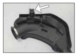
19. Remove the intake plenum mounting grommet from the intake plenum.
