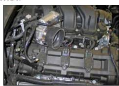
15. Install the provided silicone hose (084091) onto the throttle body and secure with the provided hose clamp.
