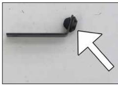
20. Install the mounting grommet from the intake plenum into the provided tube bracket as shown.
