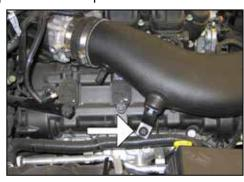
21. Install the K&N® intake tube into the silicone hump hose and then into the throttle body silicone hose. Install the tube bracket onto the mounting stud and secure it to the K&N® intake tube with the provided hardware. Tighten the hose clamps at this time.
