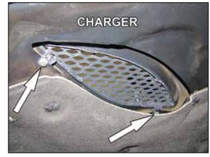
25. On vehicles equipped with hood vents: If the vehicle is to be driven during inclement weather it is recommended the shield be installed onto the hood vent to guard, the air filter from concentrated water. Remove the two bolts that secure the factory vent grid.
