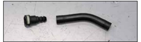
19. Remove the quick disconnect fitting from the factory flexible crank case vent line.
