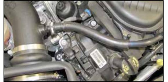
20. Install the factory quick disconnect fitting into the provided crank case vent hose and then install the assembly onto the factory hardline and connect the quick disconnect fitting to the fitting installed into the K&N® intake tube.
