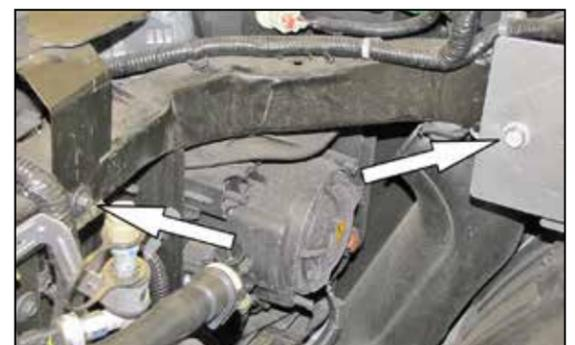
6. Remove the two factory bolts shown.
