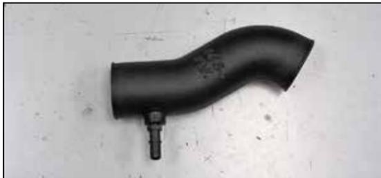
15. Install the provided quick disconnect fitting into the K&N® intake tube as shown.
