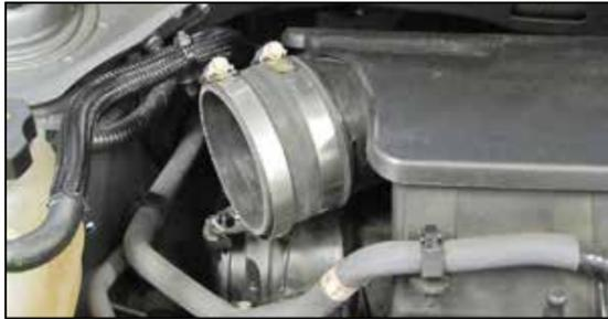
14. Install the provided coupler hose (08690) onto the intake plenum and secure with the provided hose clamp.
