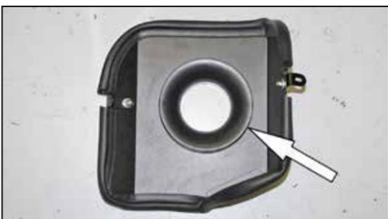
11. Install the filter adapter into the heat shield and secure with the provided hardware.
