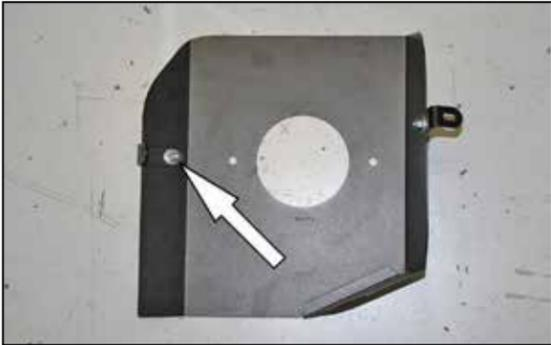
8. Install the heat shield mounting bracket (070712) onto the heat shield as shown using the provided hardware.
