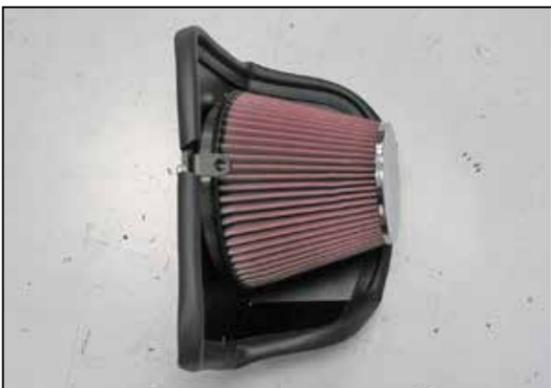
12. Install the K&N® air filter onto the filter adapter and secure with the provided hose clamp.
