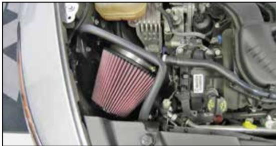
13. Install the heat shield assembly into the vehicle and secure with the hardware removed in step #6.
