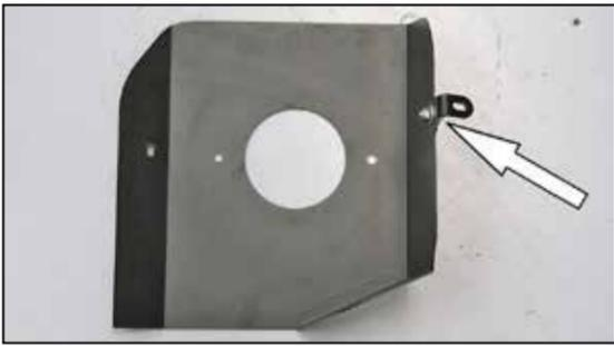
7. Install the heat shield mounting bracket (064323) onto the heat shield as shown using the provided hardware.
