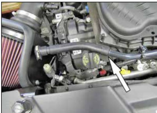
18. Remove the flexible crank case vent line from the hard line.
