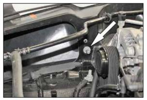
8. Remove the air filter housing mounting stud from the inner fender.
