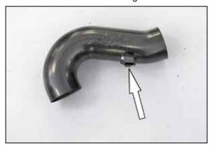
22. Install the mass air sensor into the K&N® intake tube and secure with the provided hardware.
