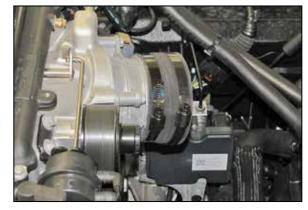
20. Install the provided coupling hose (08761) onto the throttle body and secure with the provided hose clamp.
