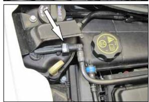
3. Release the grey locking tabs securing the crank case breather assembly to the factory intake tube and the oil tank. Then remove the crank case breather assembly from the vehicle.
