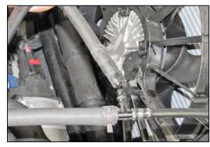
14. Cut 2" from the coolant hose and reinstall it onto the fitting and secure with the factory spring clamp.
