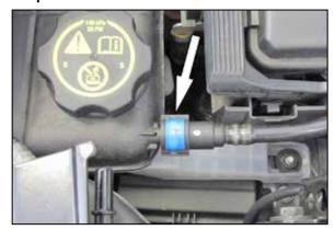
10. WARNING: Be sure the engine is completely cool before proceeding with this step! Release the blue locking tap securing the factory coolant hose to the expansion tank and then disconnect the hose from the tank.
