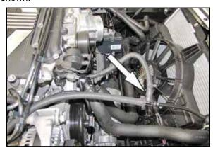
13. Release the spring clamp securing the coolant hose from the thermostat housing to the TEE fitting and then disconnect the hose from the TEE fitting. NOTE: Be sure to collect any coolant that is lost.
