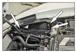
15. Install the three provided rubber mounted studs onto the air filter housing mounting locations as shown.
