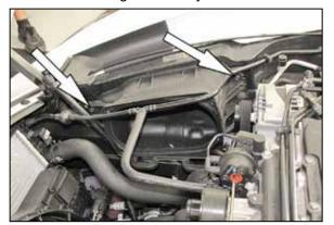
7. Remove the two bolts that secure the air filter housing to the inner fender and then remove the housing from the vehicle.
