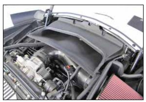
27. Reinstall the air extraction duct and secure with the provided hardware.
