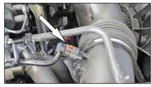
4. Release the red locking tab securing the mass air sensor electrical connection and then disconnect the mass air sensor electrical connection.
