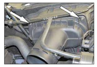
6. Loosen the two screws that secure the mass air sensor housing the air filter housing and then remove the housing and factory air filter.
