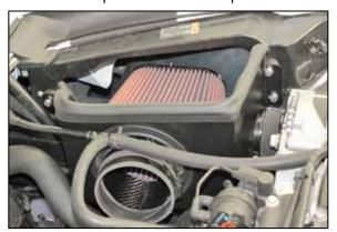
19. Install the heat shield/filter assembly onto the rubber mounted studs installed during step #13 and secure with the provided hardware.
