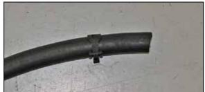
9. Assemble the coolant hose (08636), spring clamp and quick disconnect fitting as shown and then install the other spring clamp 1.5" from the open end of the hose as shown.
