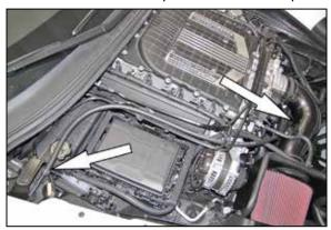
25. Install the provided crank case breather hose onto the fitting on the oil tank and then onto the fitting on the K&N® intake tube and secure with the provided spring clamps. Secure the hose as shown with the provided tie wraps.
